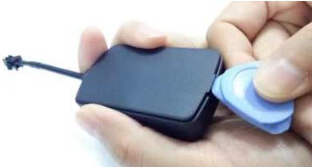
Figure 6. Opening the Case
