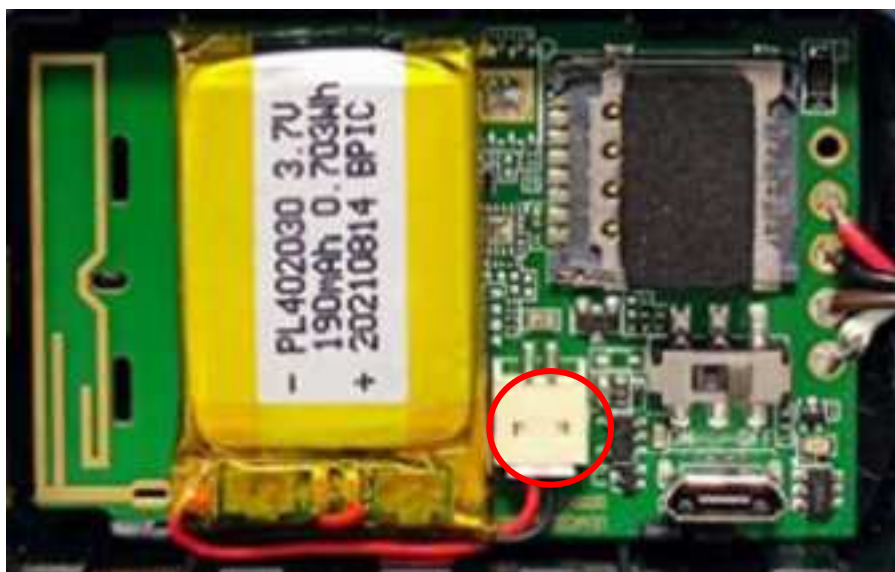
Figure 9. Installing the Internal Backup Battery
