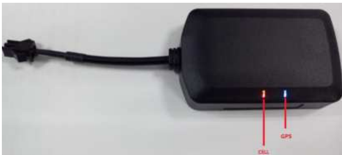
Figure 12. GV50(P) LEDs on the Case
