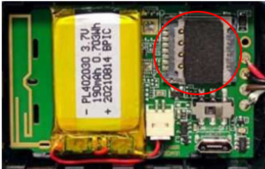
Figure 8. Installing a SIM Card
