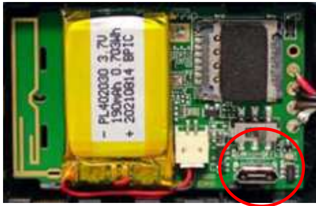
Figure 5. GV50(P) Micro USB Connector
