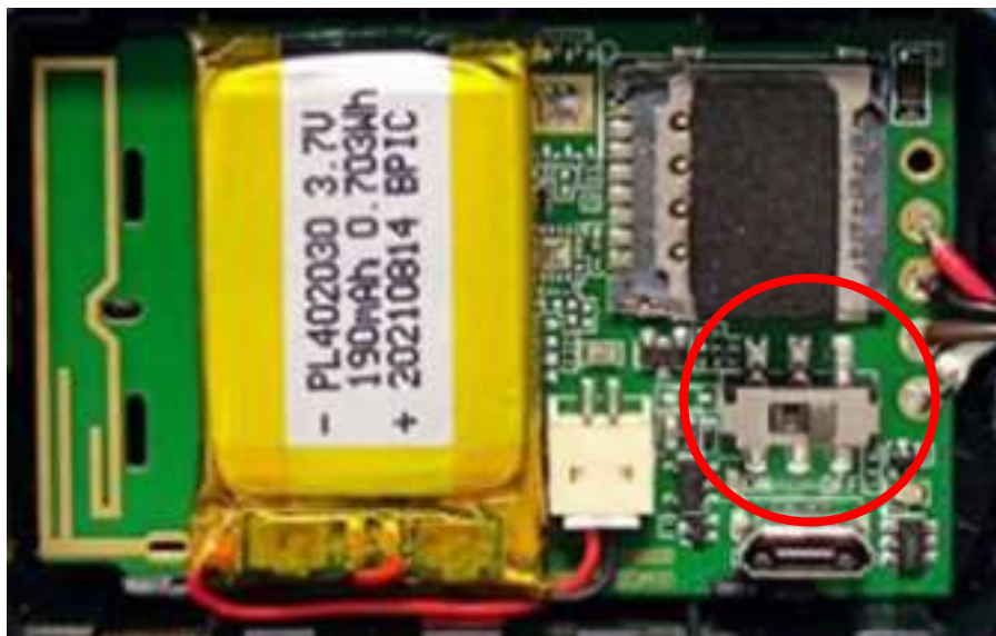
Figure 10. Switch and ON/OFF Position
