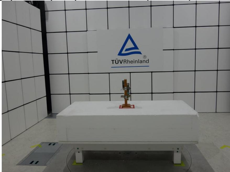
**Photograph 2: Set-up for Spurious Emissions (Back View 1)**
