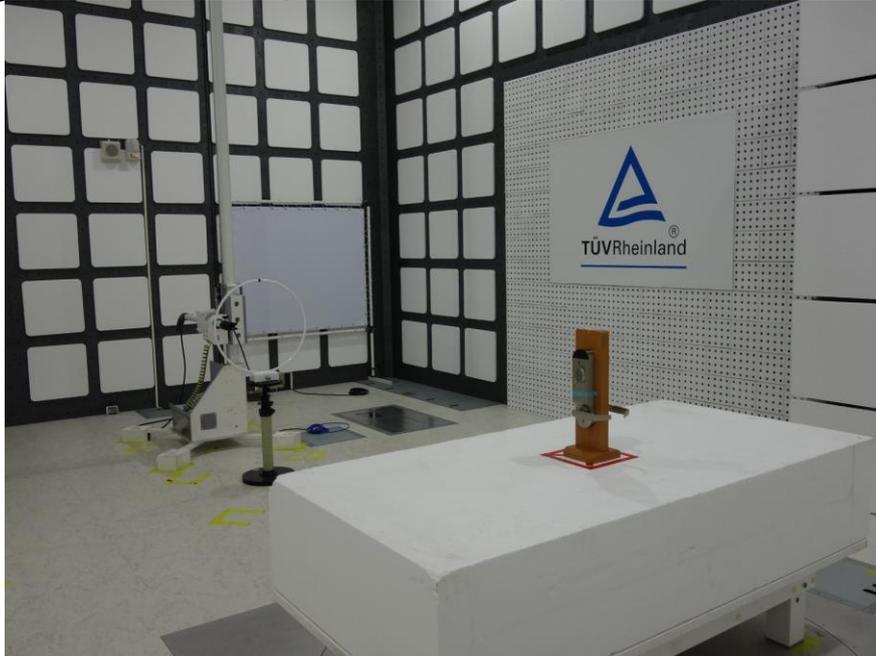
**Photograph 6: Set-up for Spurious Emissions (Back View 5)**
