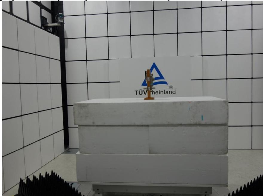
**Photograph 4: Set-up for Spurious Emissions (Back View 3)**
