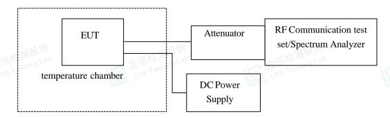
Frequency Stability vs. Temperature: The equipment under test was connected to an external DC power supply and the RF output was connected to a Frequency Counter via feed-through attenuators. The EUT was placed inside the temperature chamber. The DC leads and RF output cable exited the chamber through an opening made for the purpose.
