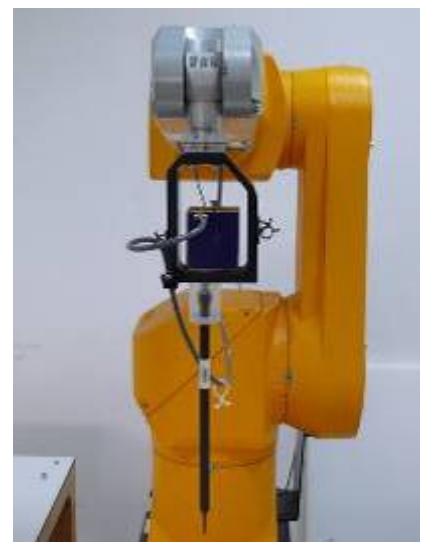
Figure 3. EX3DV4 E-field probe
