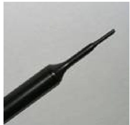
Figure 2. EX3DV4 E-field Probe
