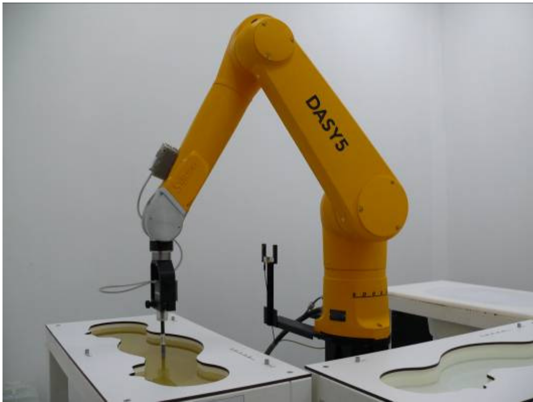
Picture 1: Specific Absorption Rate Test Layout
