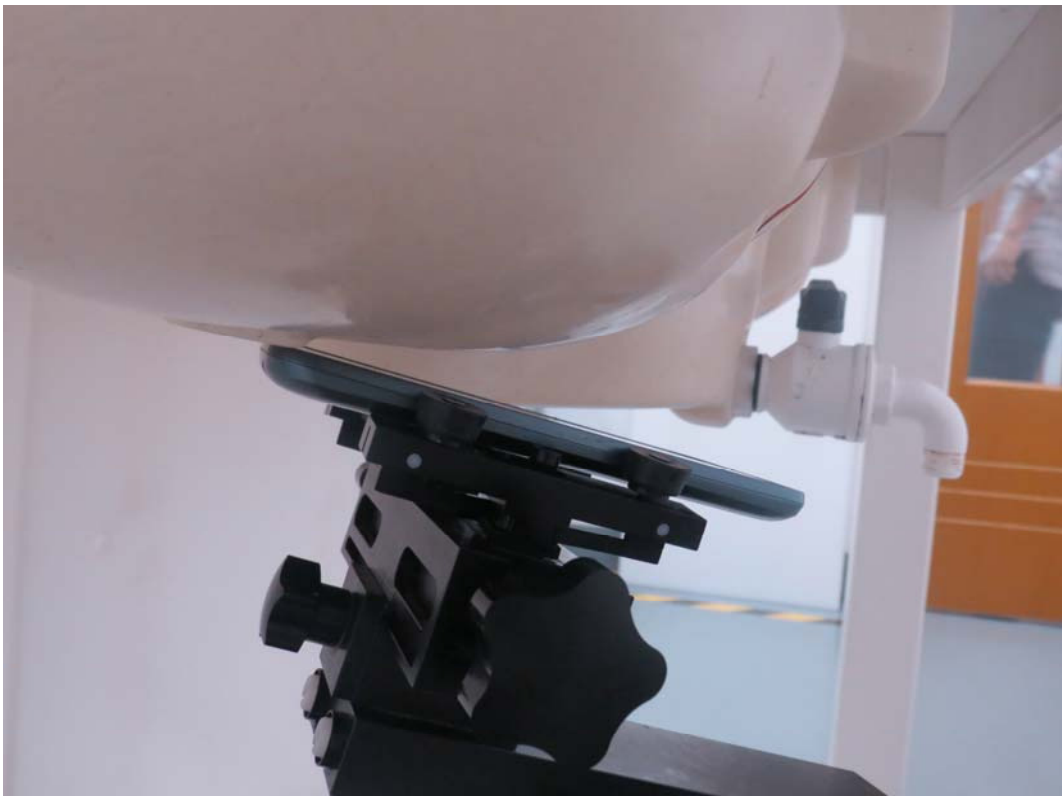
Picture 18: Right Hand Tilt 15 Degree Position (7040T)
