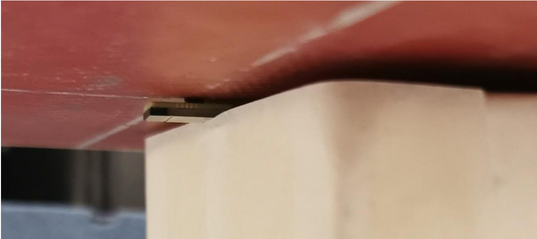
Figure 13 Back test position, RF Energy Enhancement, 0mm separation distance
