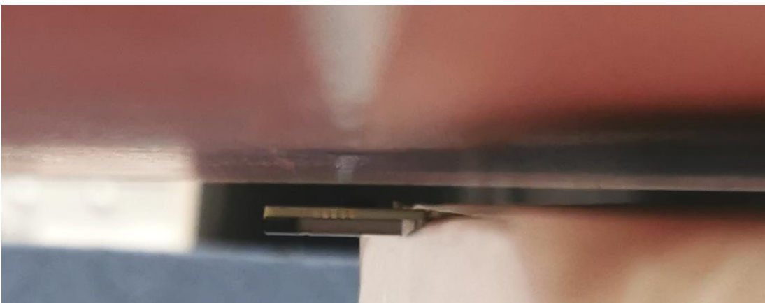
Figure 14 Back test position, RF Energy Enhancement, 5mm separation distance
