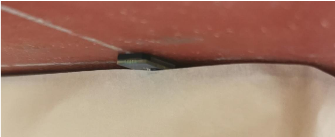
Figure 10 Front test position, RF Energy Coupling Enhancement, 0mm separation distance
