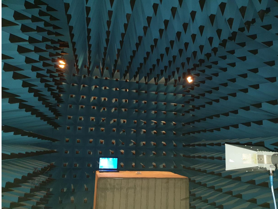
Radiated Test Picture(Front) _Above 1GHz
