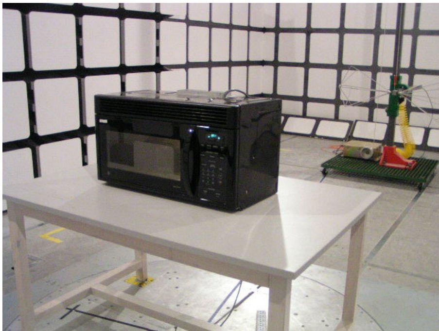
30MHz to 1000MHz: Radiated Emission - Front View
