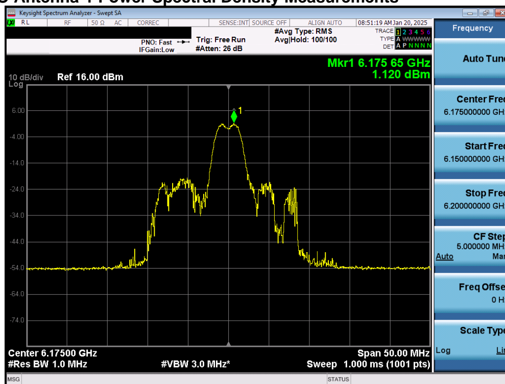
Plot 7-33. Power Spectral Density Plot MIMO ANT1 (20MHz 802.11ax (26 Tones) (UNII Band 5) – Ch. 45) - LPI
