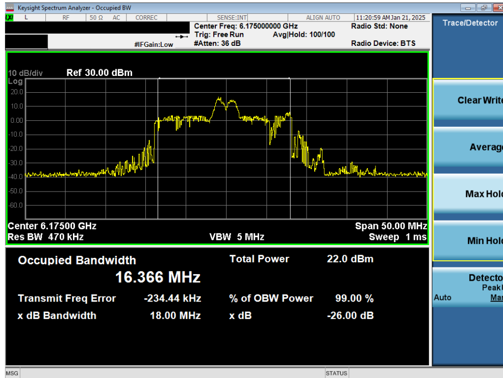
Plot 7-21. 26dB Bandwidth Plot MIMO ANT2 (20MHz 802.11ax (26 Tones) (UNII Band 5) – Ch. 45) - SP
