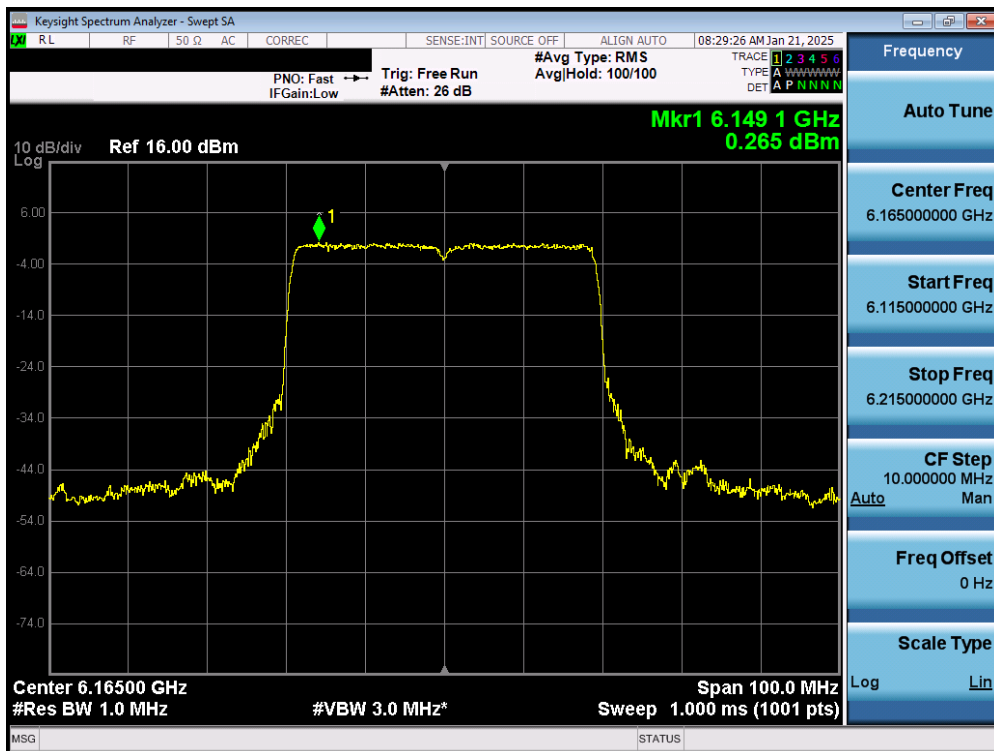
Plot 7-46. Power Spectral Density Plot MIMO ANT1 (40MHz 802.11ax (Full Tones) (UNII Band 5) – Ch. 43) - SP
