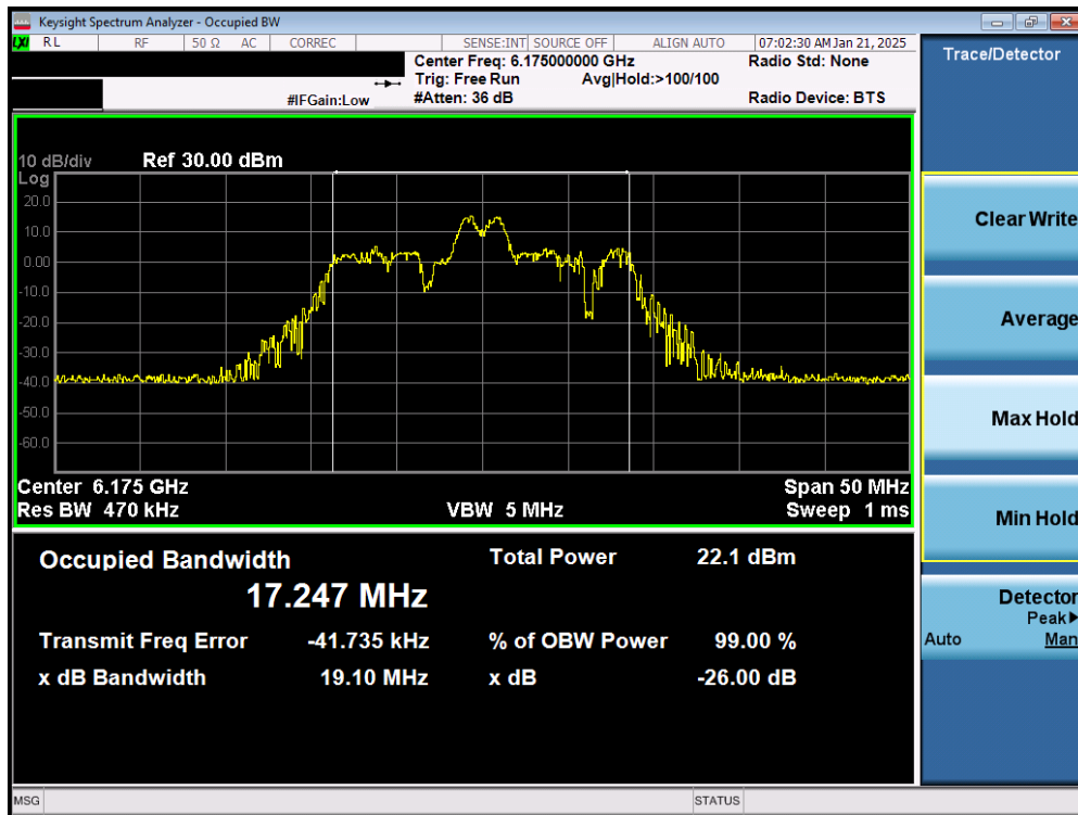
Plot 7-5. 26dB Bandwidth Plot MIMO ANT1 (20MHz 802.11ax (26 Tones) (UNII Band 5) – Ch. 45) – SP
