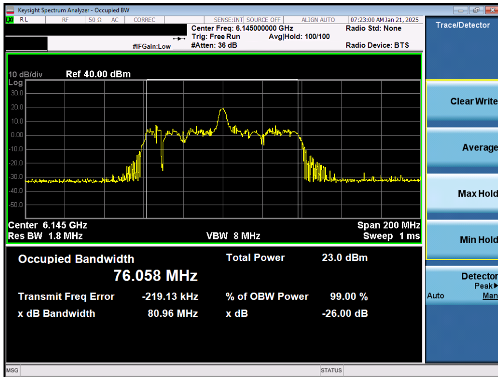
Plot 7-7. 26dB Bandwidth Plot MIMO ANT1 (80MHz 802.11ax (26 Tones) (UNII Band 5) – Ch. 39) - SP
