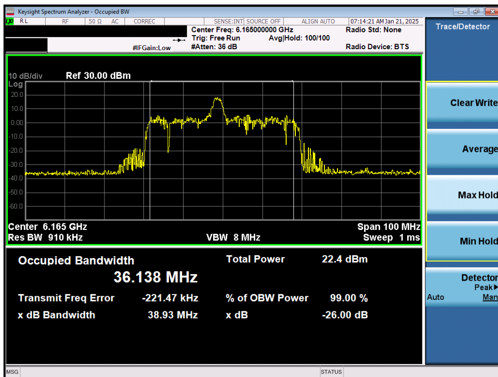
Plot 7-6. 26dB Bandwidth Plot MIMO ANT1 (40MHz 802.11ax (26 Tones) (UNII Band 5) – Ch. 43) – SP
