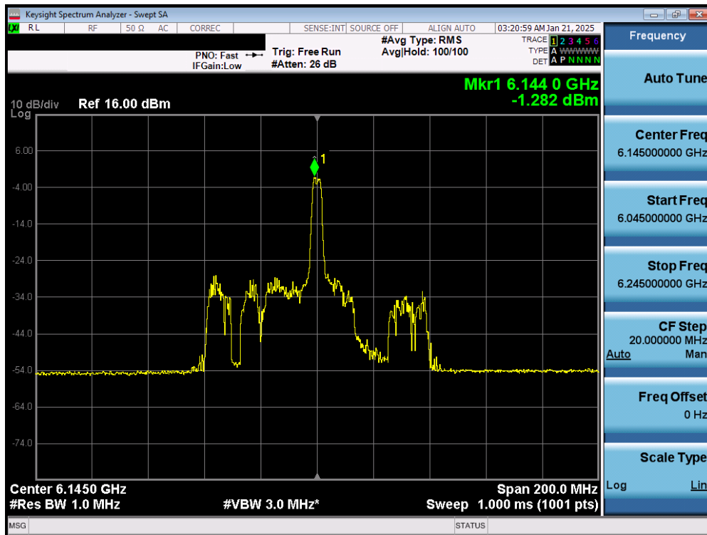
Plot 7-35. Power Spectral Density Plot MIMO ANT1 (80MHz 802.11ax (26 Tones) (UNII Band 5) – Ch. 39) - LPI
