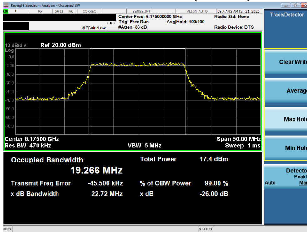
Plot 7-25. 26dB Bandwidth Plot MIMO ANT2 (20MHz 802.11ax (Full Tones) (UNII Band 5) – Ch. 45) - LPI
