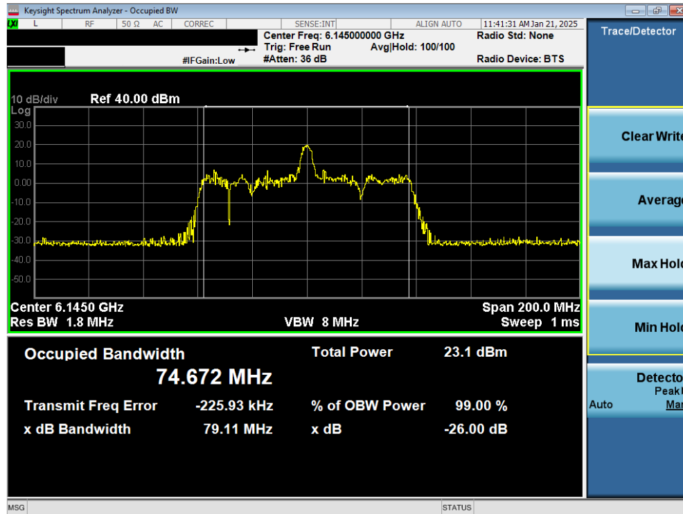
Plot 7-23. 26dB Bandwidth Plot MIMO ANT2 (80MHz 802.11ax (26 Tones) (UNII Band 5) – Ch. 39) - SP
