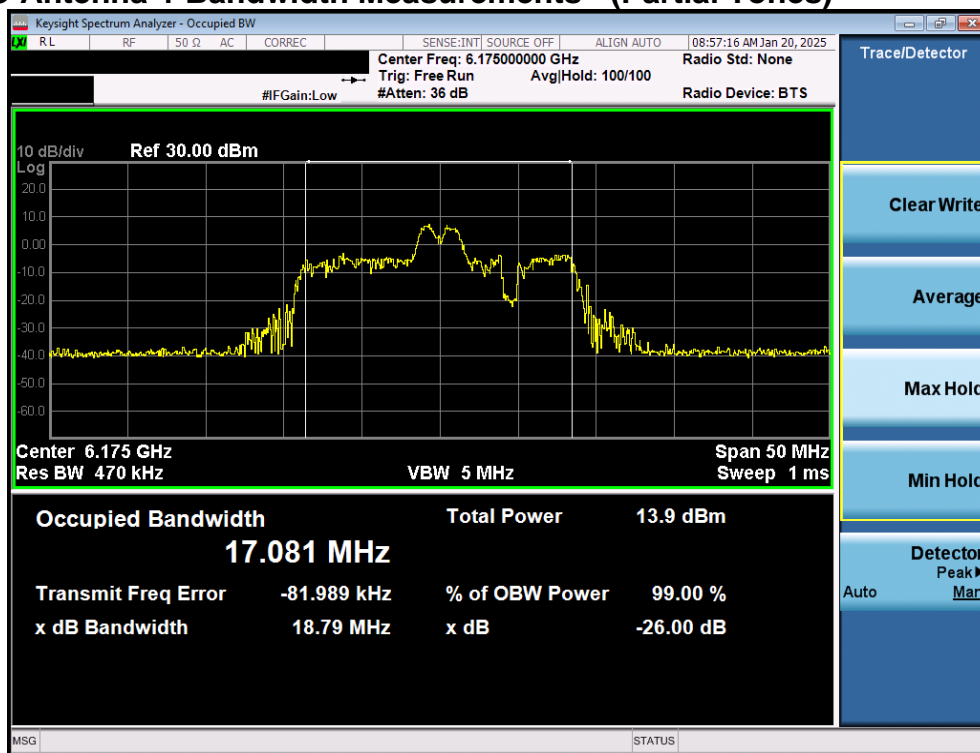
Plot 7-1. 26dB Bandwidth Plot MIMO ANT1 (20MHz 802.11ax (26 Tones) (UNII Band 5) – Ch. 45) - LPI
