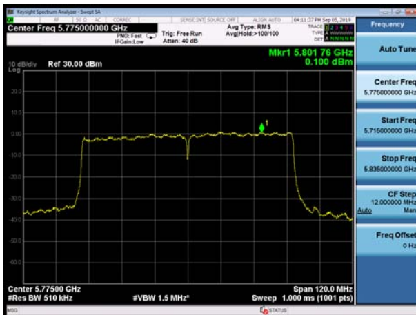
U-NII-3, 802.11ac VHT80, Channel No.: 155
