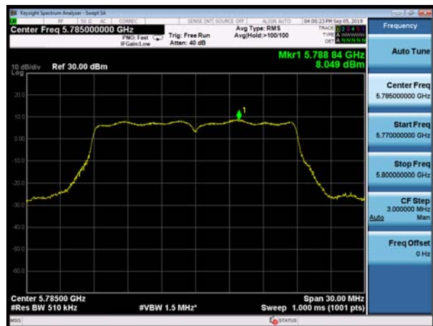
U-NII-3, 802.11ac VHT20, Channel No.: 165
