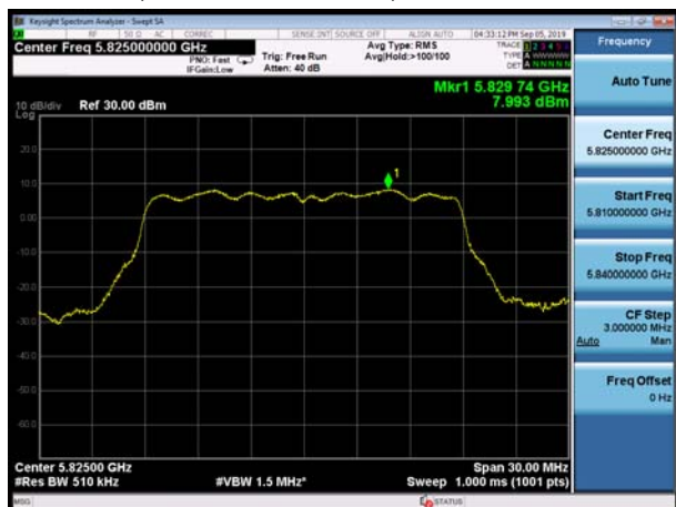
U-NII-3, 802.11ac VHT20, Channel No.: 165
