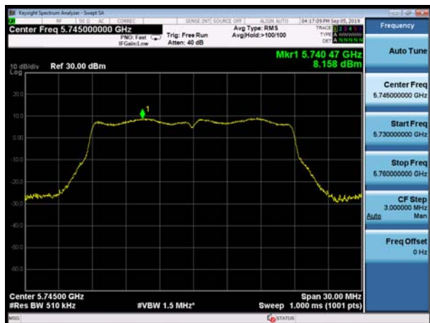
U-NII-3, 802.11ac VHT20, Channel No.: 157
