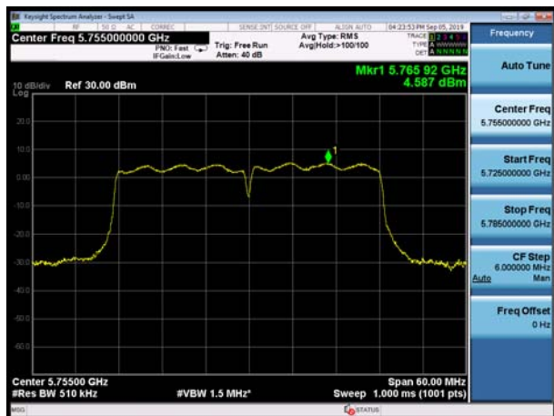
U-NII-3, 802.11ac VHT40, Channel No.: 159
