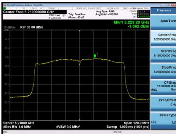
U-NII-1, 802.11ac VHT80, Channel No.: 42
