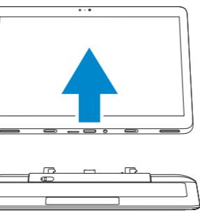
NOTE: Undock the computer to access SIM card slot.
