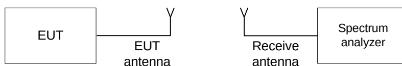
Figure 7.3.1 Hopping frequencies test setup
