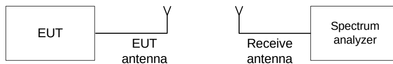
Figure 7.2.1 Carrier frequency separation test setup
