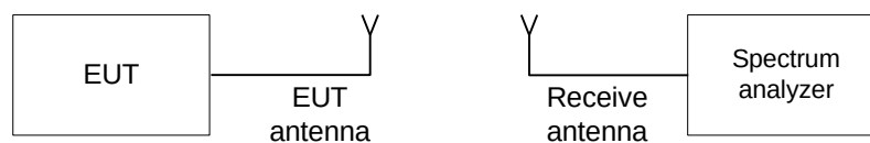
Figure 7.1.1 The 20 dB bandwidth test setup
