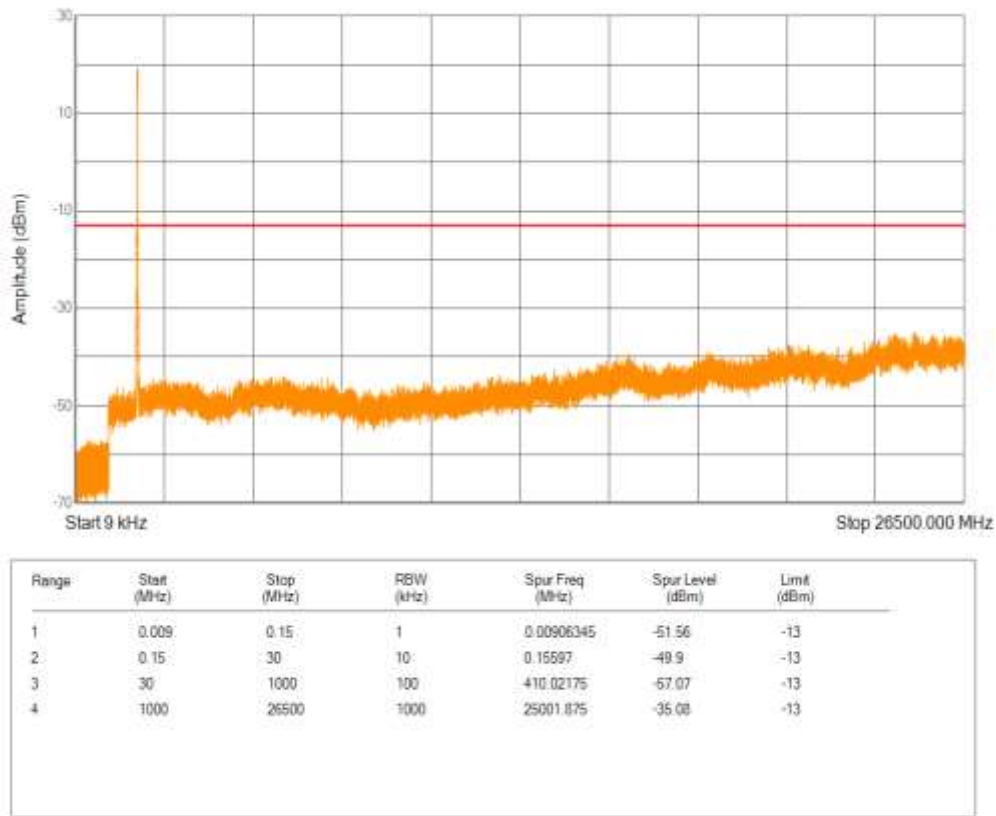
Band25 QAM16 BW=15MHz Channel=26115 RB Size=75 Position=#0
