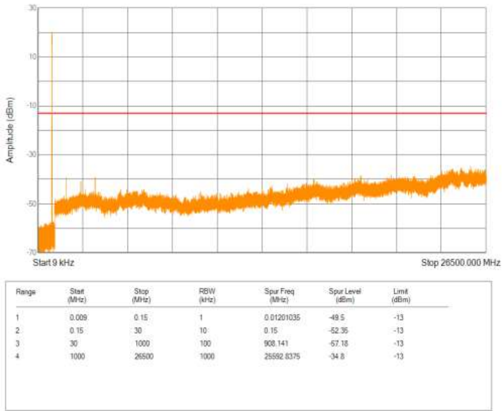
Band26(824-849) QPSK BW=3MHz Channel=26805 RB Size=15 Position=#0
