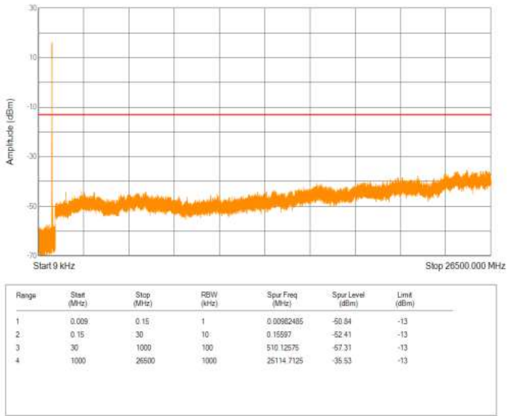
Band26(814-824) QPSK BW=3MHz Channel=26775 RB Size=15 Position=#0
