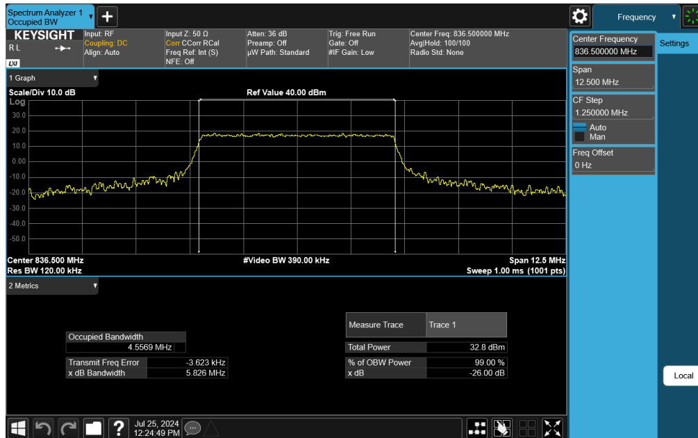
Plot 7-11. Occupied Bandwidth Plot (LTE Band 26/5 - 5MHz 64-QAM - Full RB Configuration)
