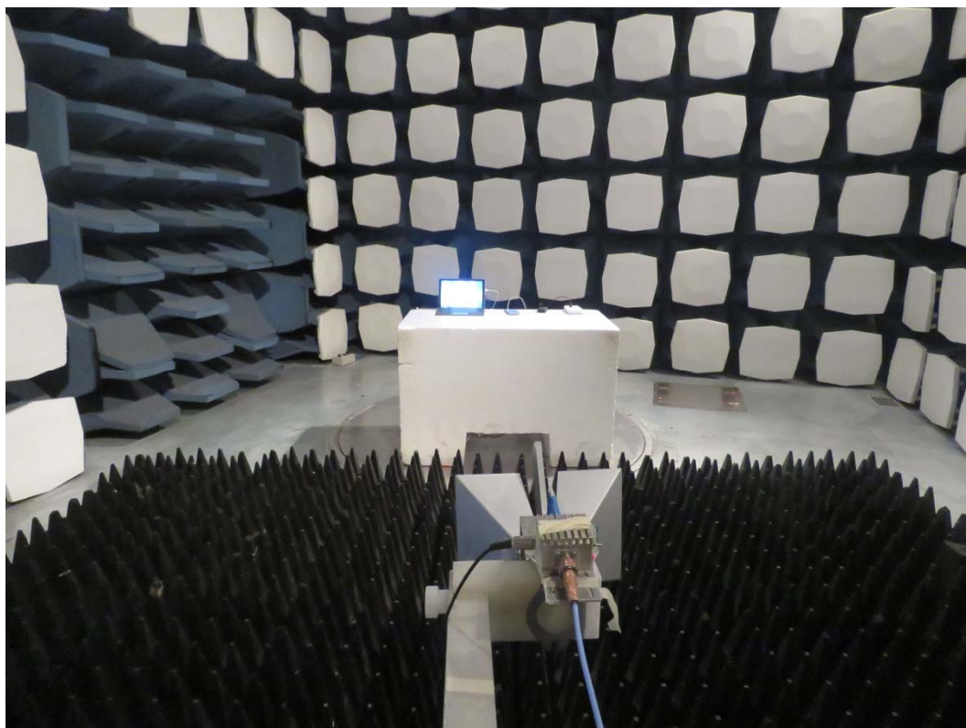
Picture 1: Radiated Emission Test Setup
