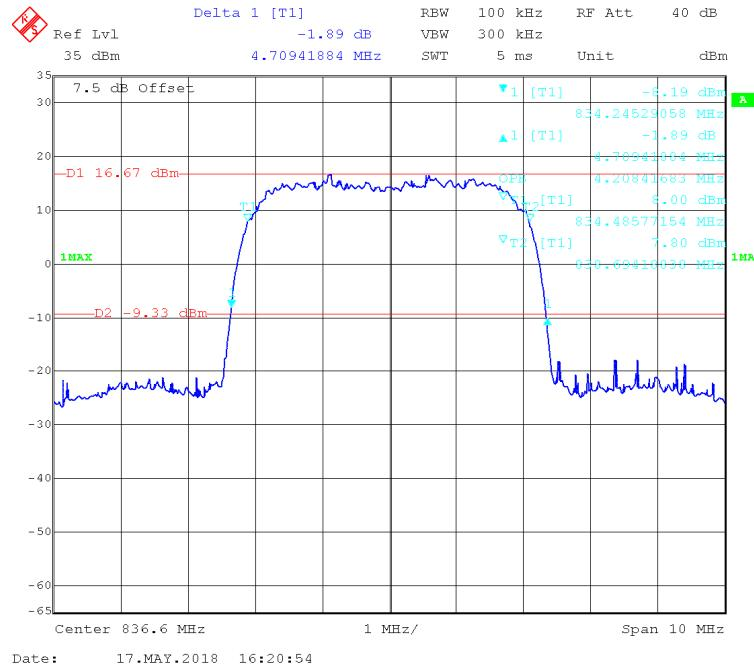
**99% Occupied & 26 dB Emissions Bandwidth for WCDMA (HSDPA) Mode**
