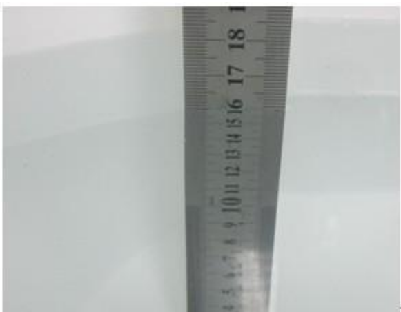
Liquid Height for Body SAR
