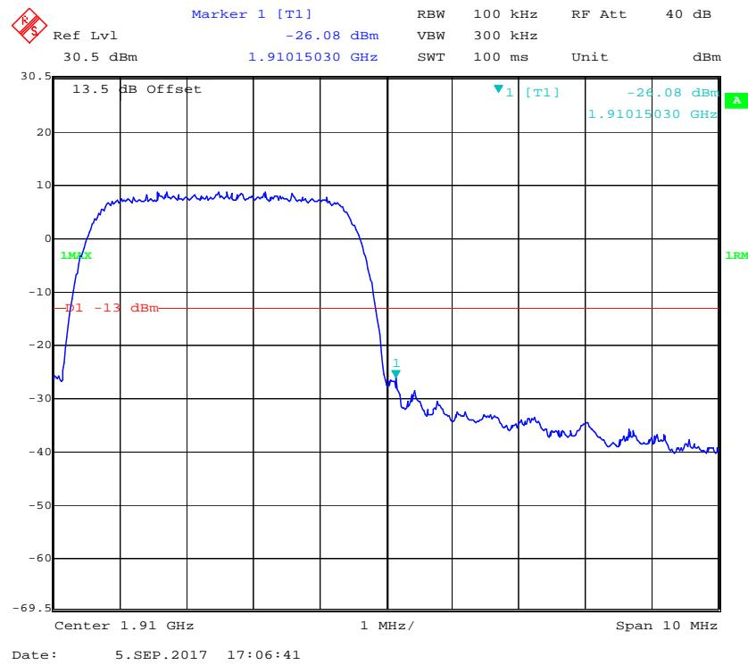
**PCS Band, Left Band Edge for HSUPA (BPSK) Mode**
