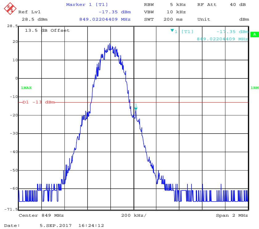
**Cellular Band, Left Band Edge for RMC (BPSK) Mode**
