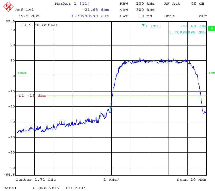
**AWS Band, Right Band Edge for HSUPA (BPSK) Mode**
