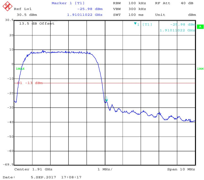
**AWS Band, Left Band Edge for RMC (BPSK) Mode**
