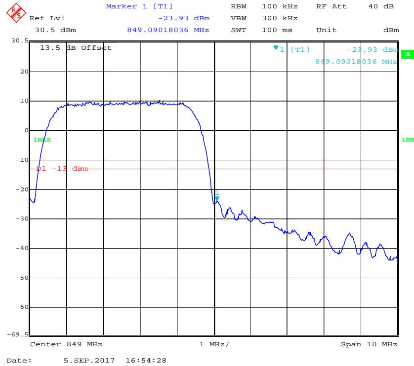
**Cellular Band, Left Band Edge for HSDPA (16QAM) Mode**
