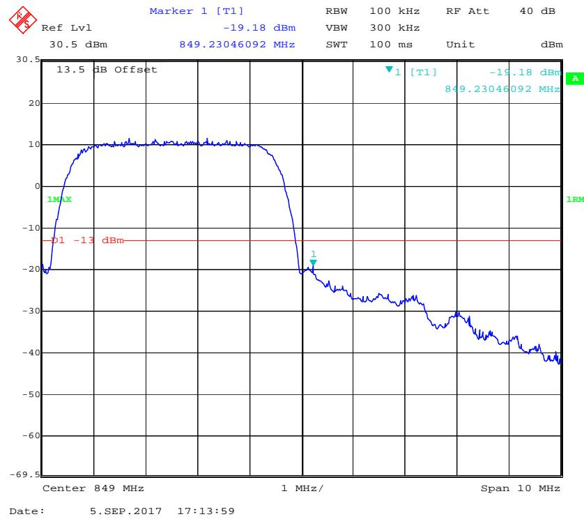
**PCS Band, Left Band Edge for GSM (GMSK) Mode**
