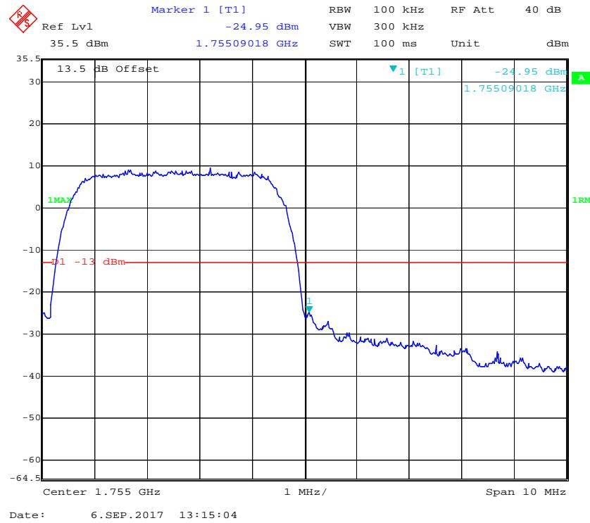
**AWS Band, Left Band Edge for HSUPA (BPSK) Mode**
