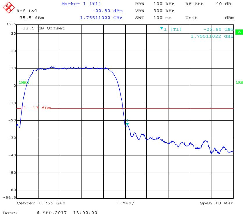
**AWS Band, Left Band Edge for HSDPA (16QAM) Mode**
