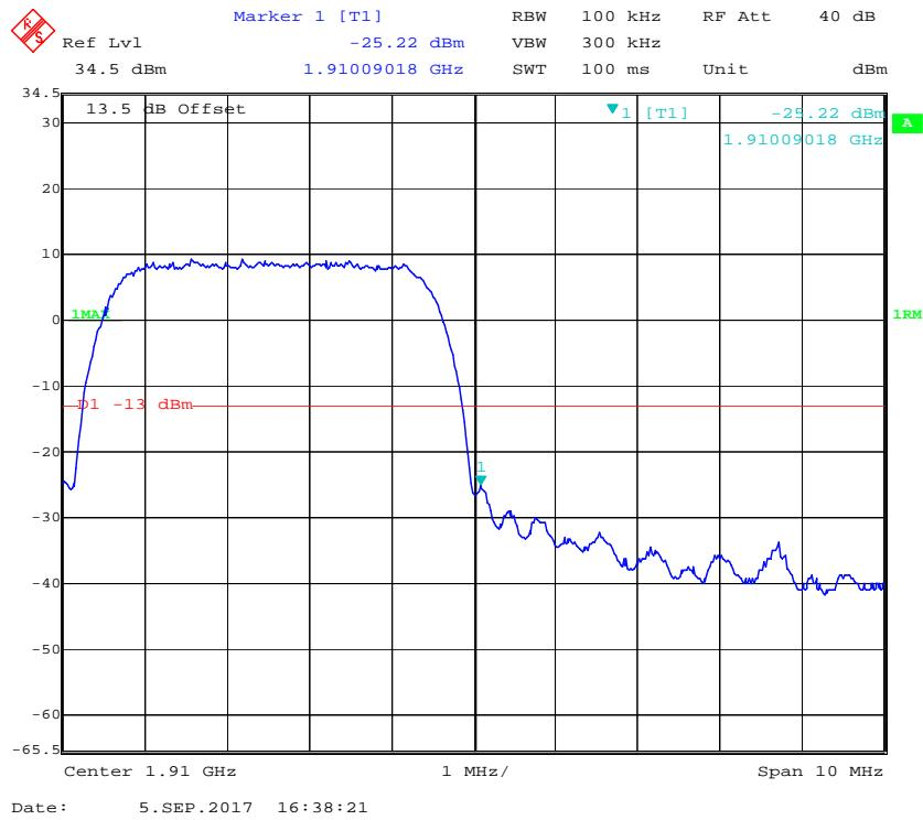
**PCS Band, Left Band Edge for HSDPA (16QAM) Mode**
