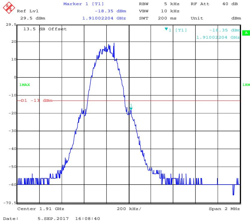
**PCS Band, Left Band Edge for RMC (BPSK) Mode**
