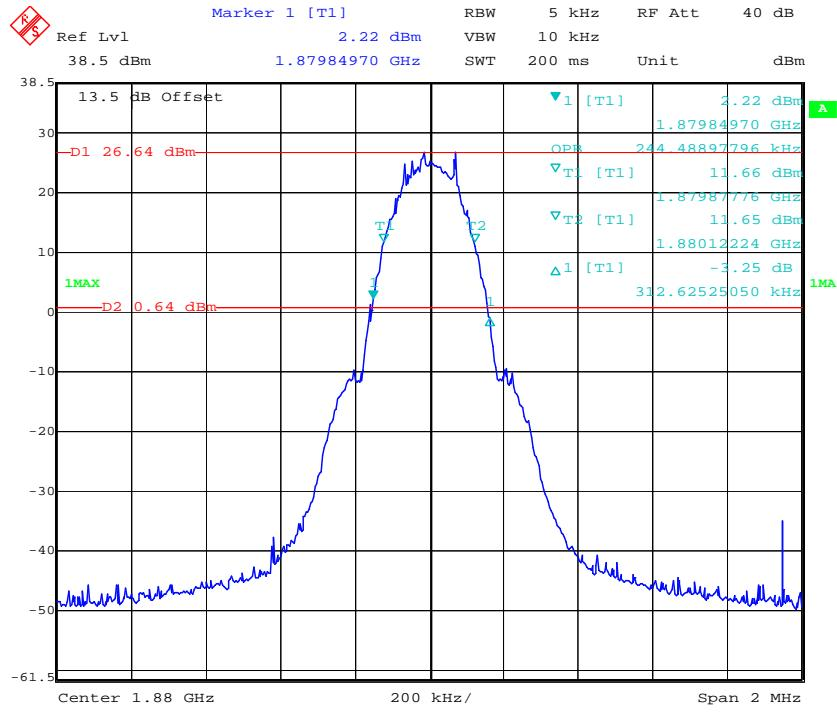
**26 dB Emissions & 99% Occupied Bandwidth for RMC (BPSK) Mode**
