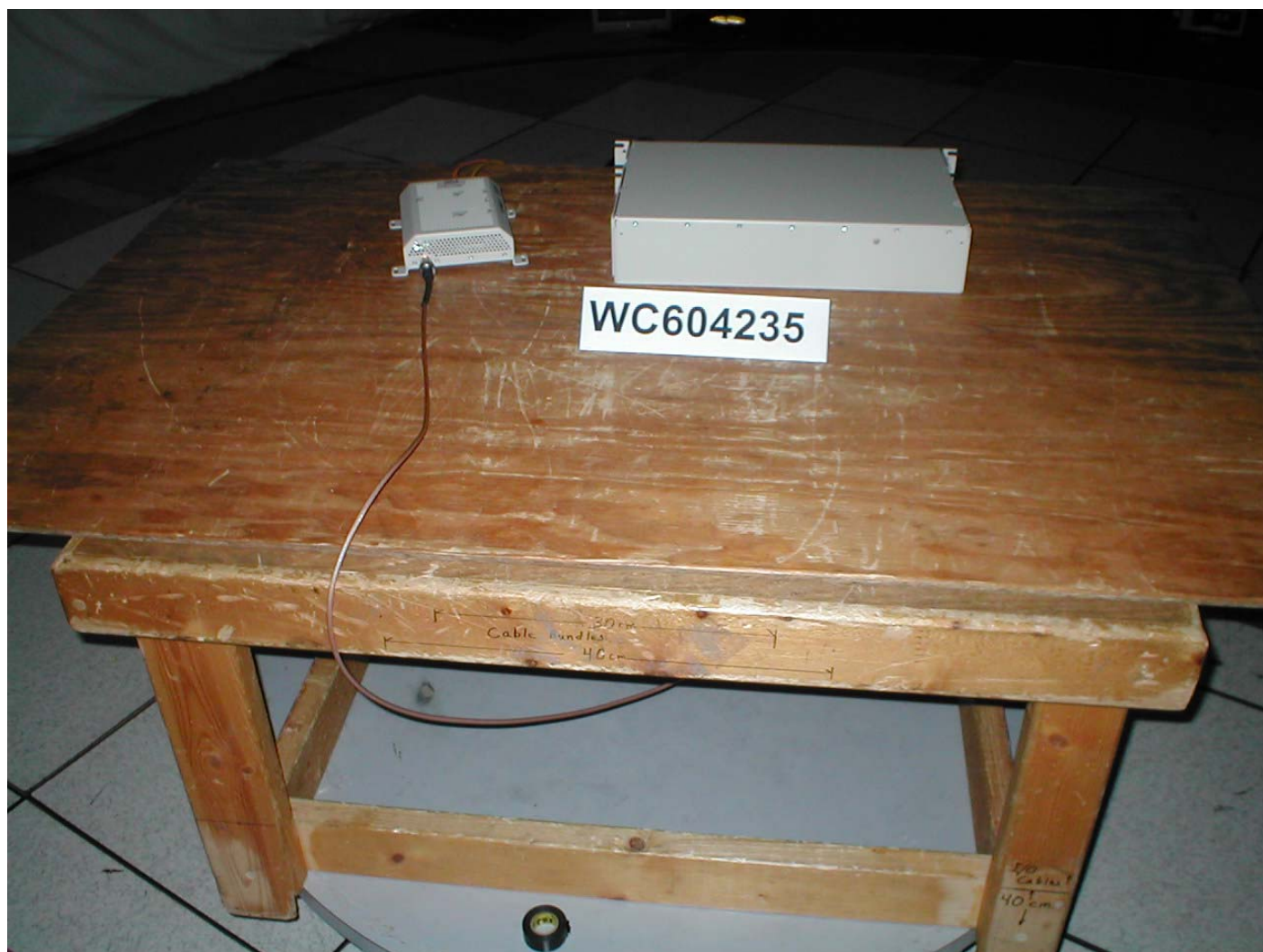
Test setup photo, radiated emissions
