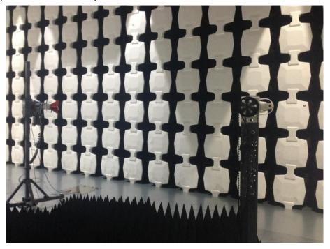
Description: Substitution Antenna for EIRP Test
