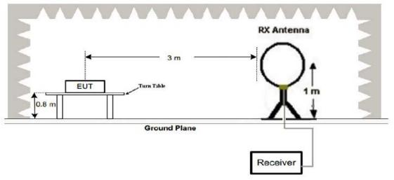
(2) Radiated Emission Test-Up Frequency 30MHz~1GHz
