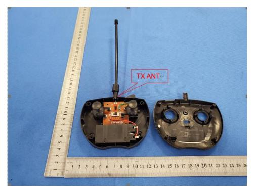
Length: 19cm Antenna Type: Spring Antenna Antenna Gain: 0dBi
