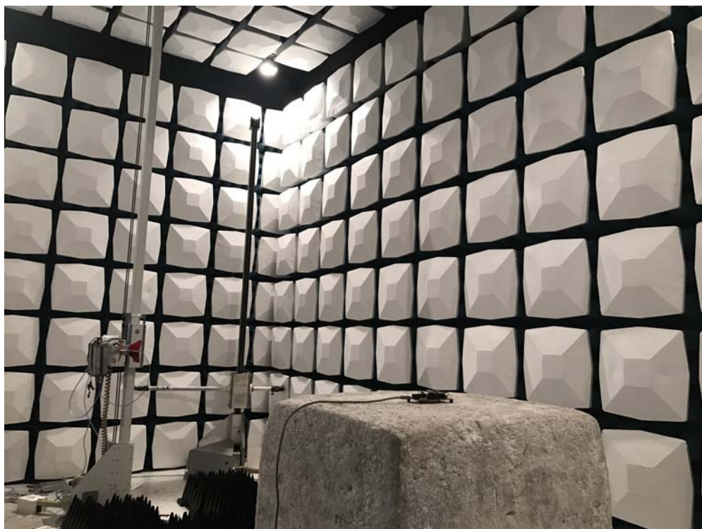
Description: Radiated Emission Test Setup for 1~18GHz
