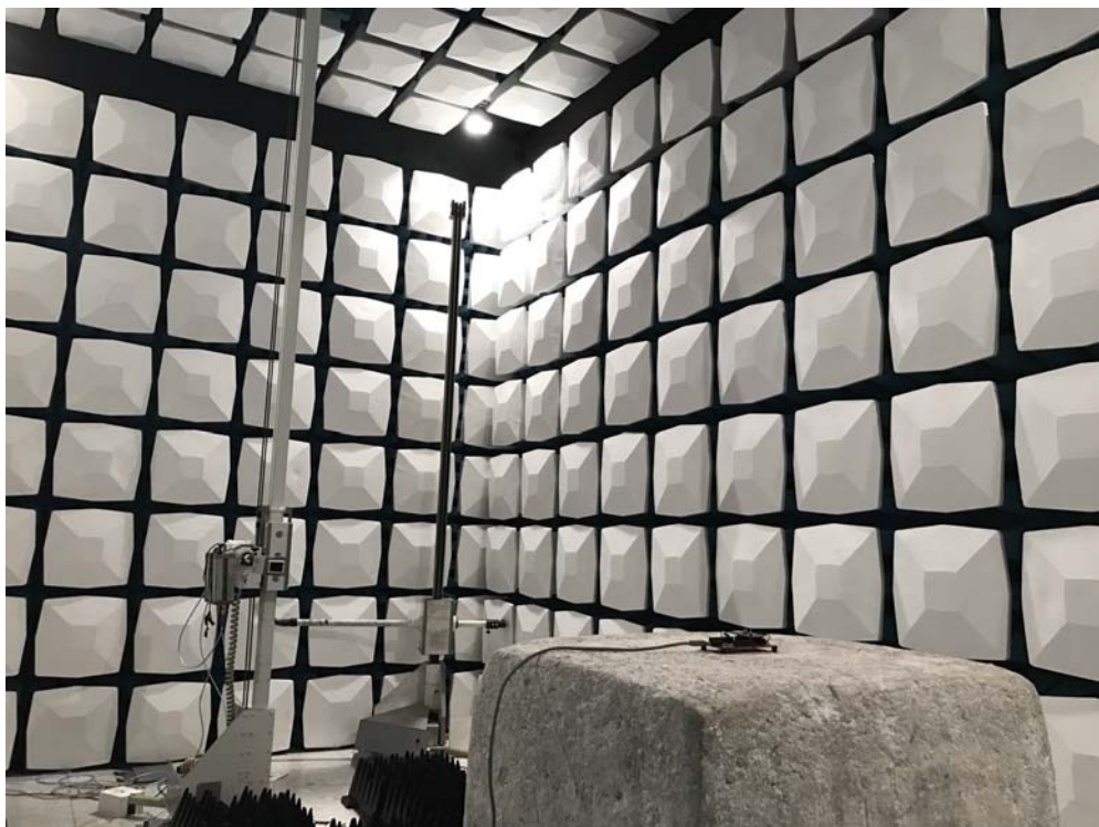
Description: Radiated Emission Test Setup for 18~40GHz
