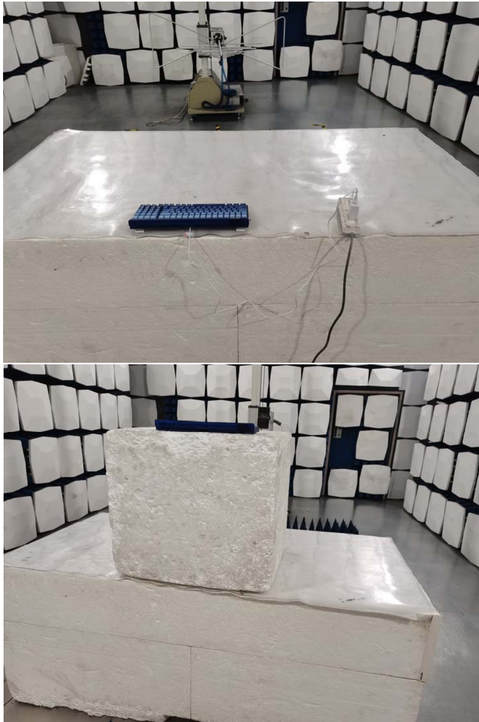
Radiated emission test view
