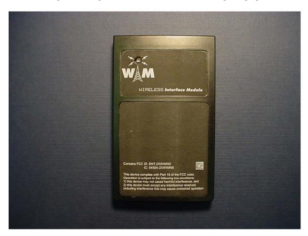
PowerFlex Wireless Interface Module 2.402 – 2.480 GHz
