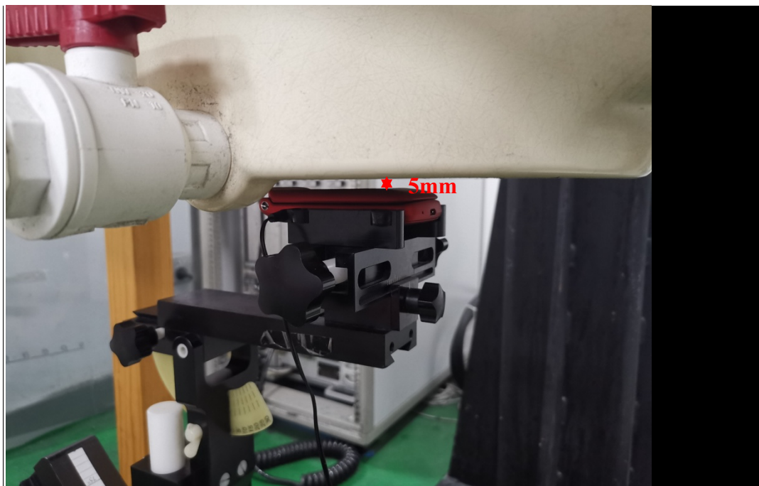
Body Worn Front Setup Photo (5mm)
