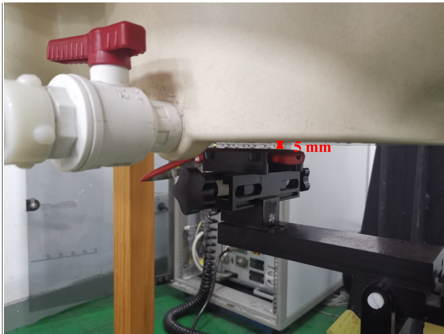
Body Worn Back Setup Photo (5mm)
