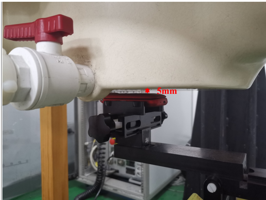
Body Worn Front Setup Photo (5mm)
