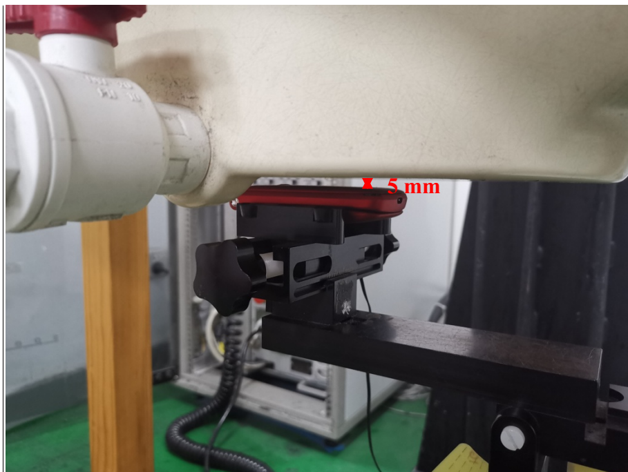
Body Worn Back Setup Photo (5mm)
