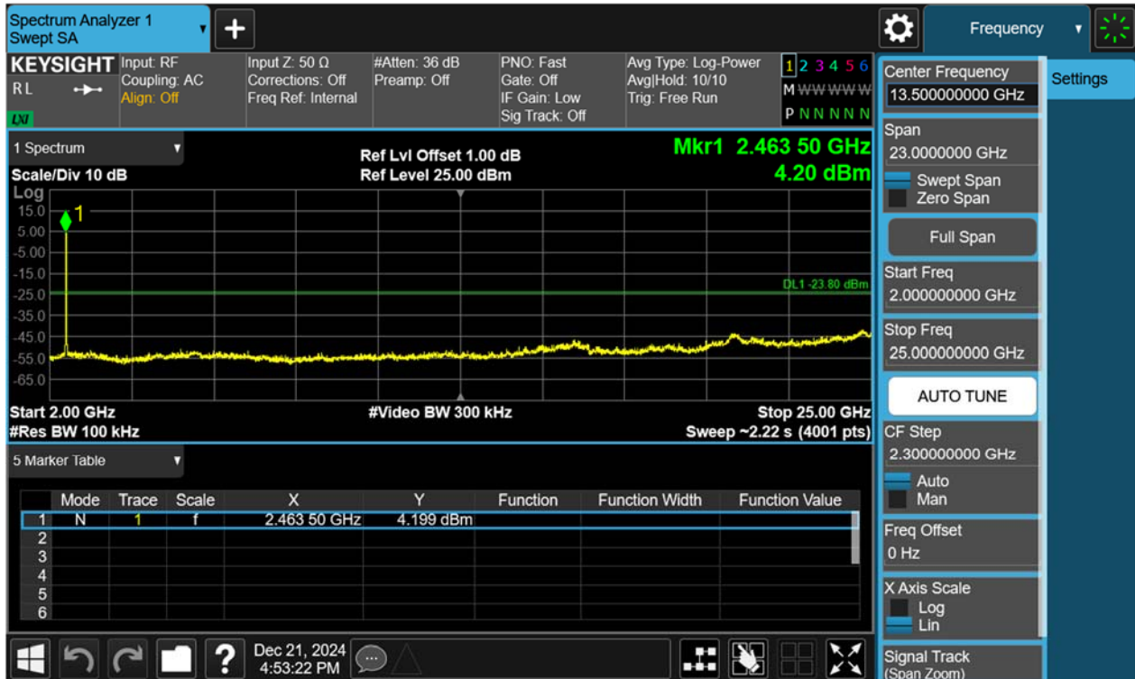
Figure 58: Conducted Spurious Emission & Authorized-band band-edge, 802.11g, 2412MHz Carrier Level
