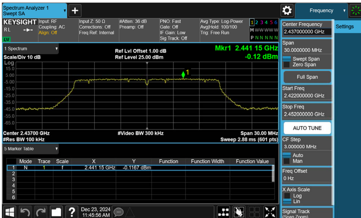
Figure 59: Conducted Spurious Emission & Authorized-band band-edge, 802.11g, 2437MHz Carrier Level
