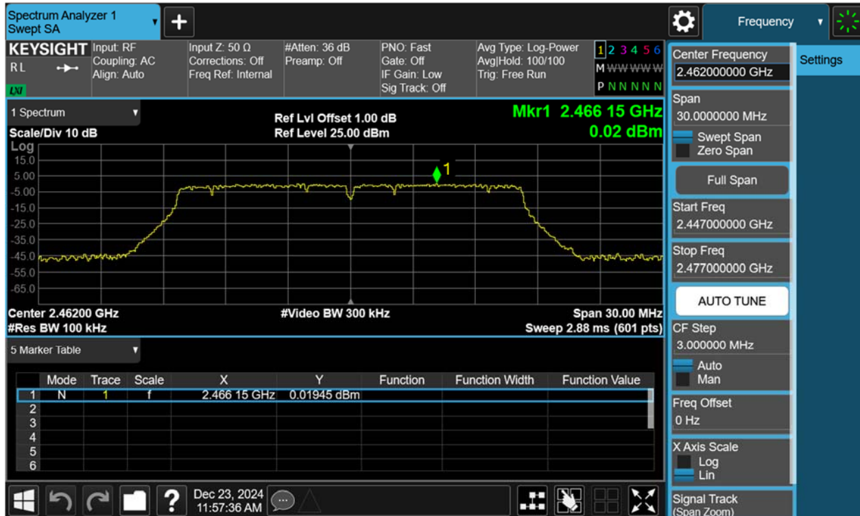
Figure 60: Conducted Spurious Emission & Authorized-band band-edge, 802.11g, 2462MHz Carrier Level
