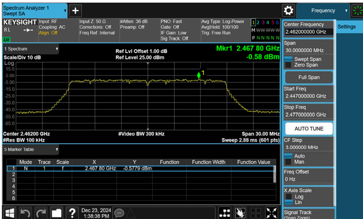
Figure 63: Conducted Spurious Emission & Authorized-band band-edge, 802.11n(HT20), 2462MHz Carrier Level
