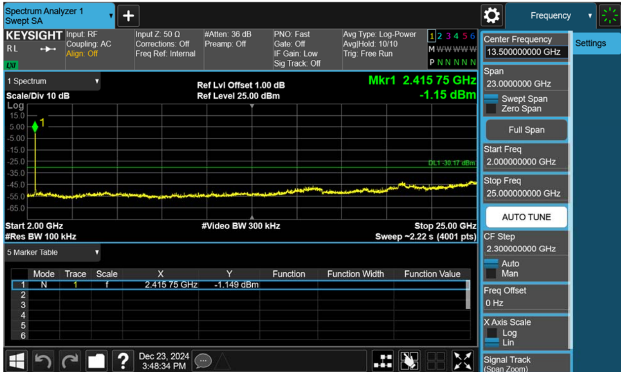
Figure 65: Conducted Spurious Emission & Authorized-band band-edge, 802.11ax(HE20), 2437MHz Carrier Level
