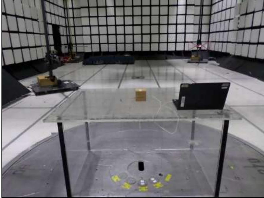
**Photograph 9. Spurious Emissions, 30MHz – 135.6MHz, Rear Setup**
