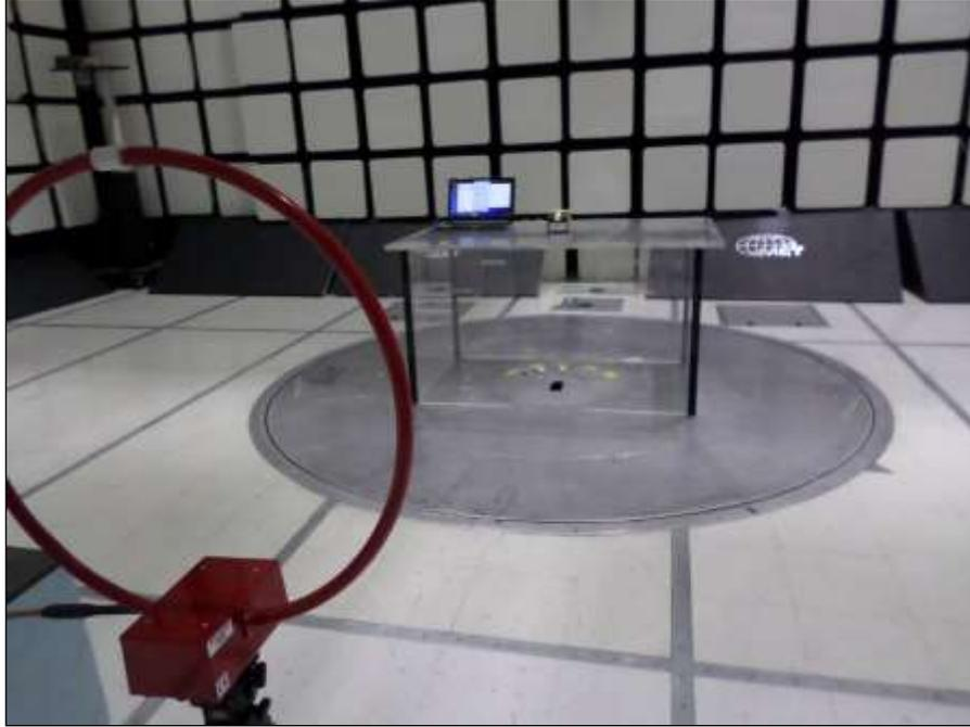
**Photograph 3. Spurious Emissions, 9KHz - 30MHz, Antenna Setup**
