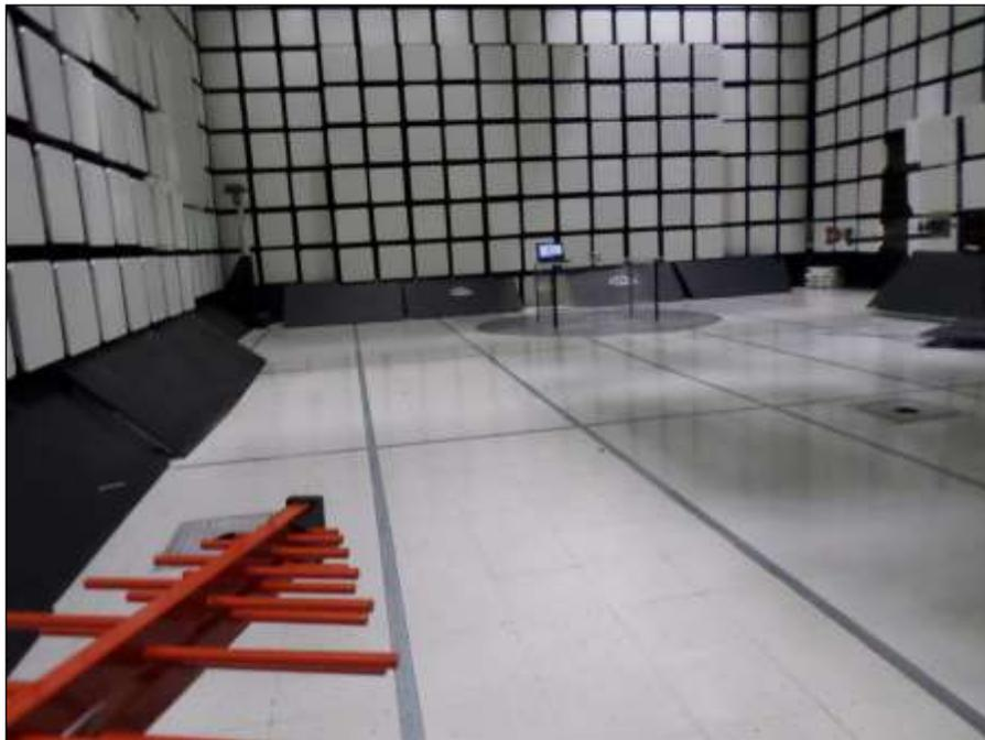
**Photograph 6. Spurious Emissions, 30MHz - 135.6MHz, Antenna Setup**
