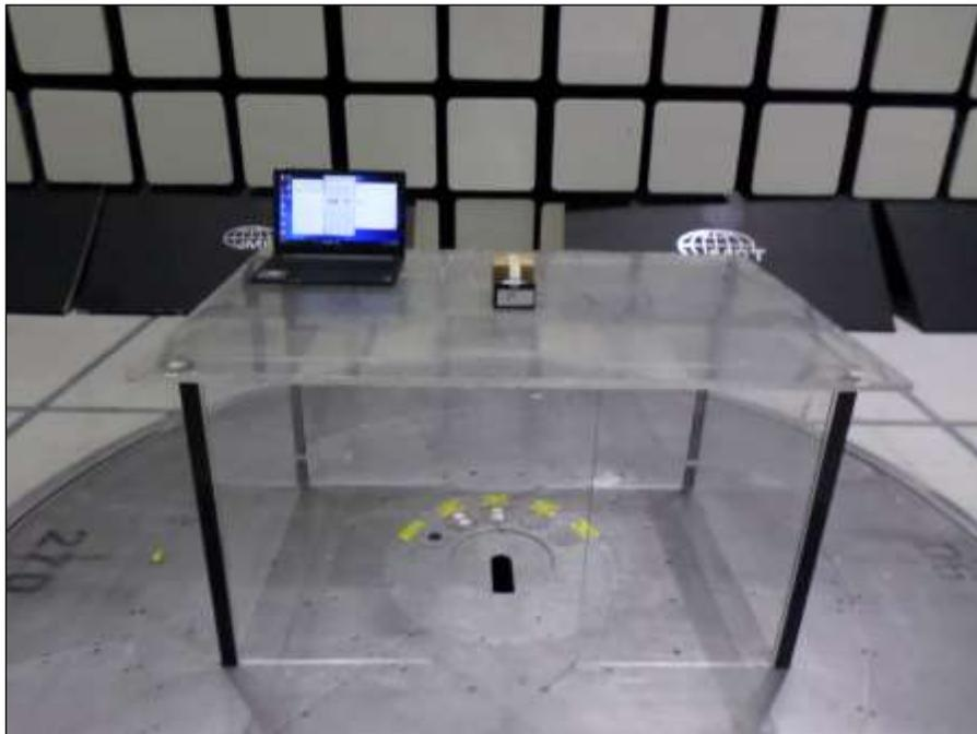
**Photograph 8. Spurious Emissions, 30MHz – 135.6MHz, Front Setup**
