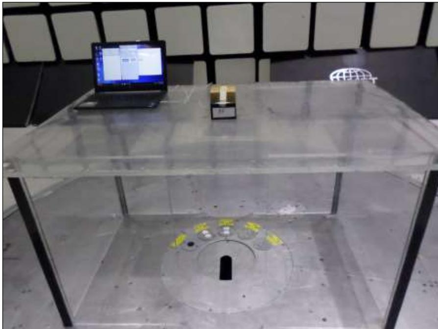
**Photograph 4. Spurious Emissions, 9KHz - 30MHz, Front Setup**
