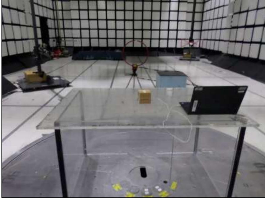
**Photograph 5. Spurious Emissions, 9KHz - 30MHz, Rear Setup**
