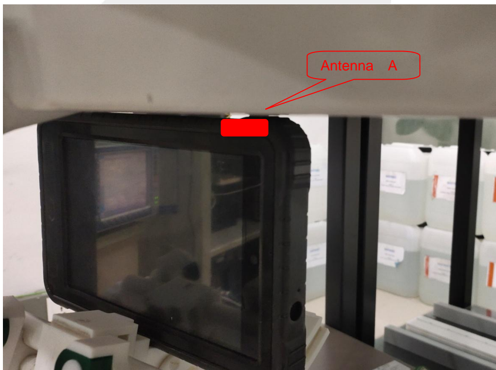
Left Edge(separation distance is 0mm)
