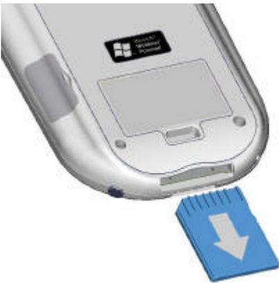
1. Push the memory card into the bottom slot until it clicks into place. The card is secure when it is not protruding from the base.
