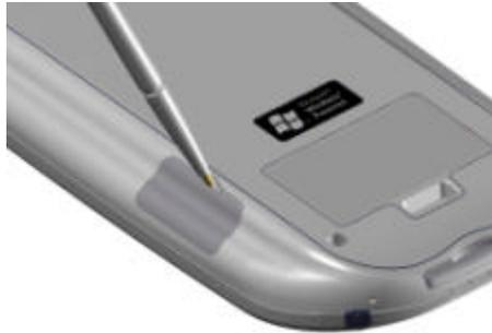
Press the point of your stylus into the hole until the Smart Card springs out; then use your fingers to finish removing.
