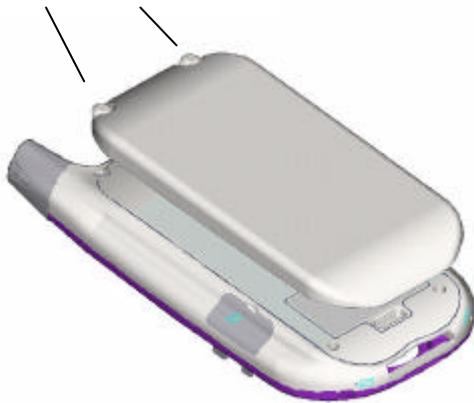
1. Remove the rubber cap protecting the Pocket PC Phone connector for the External Battery. The cap is situated just below the right screw on the back of the Pocket PC Phone.
