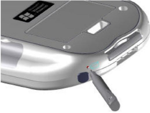
2. Press the battery switch once to turn it off, and then once more to turn it back on.
