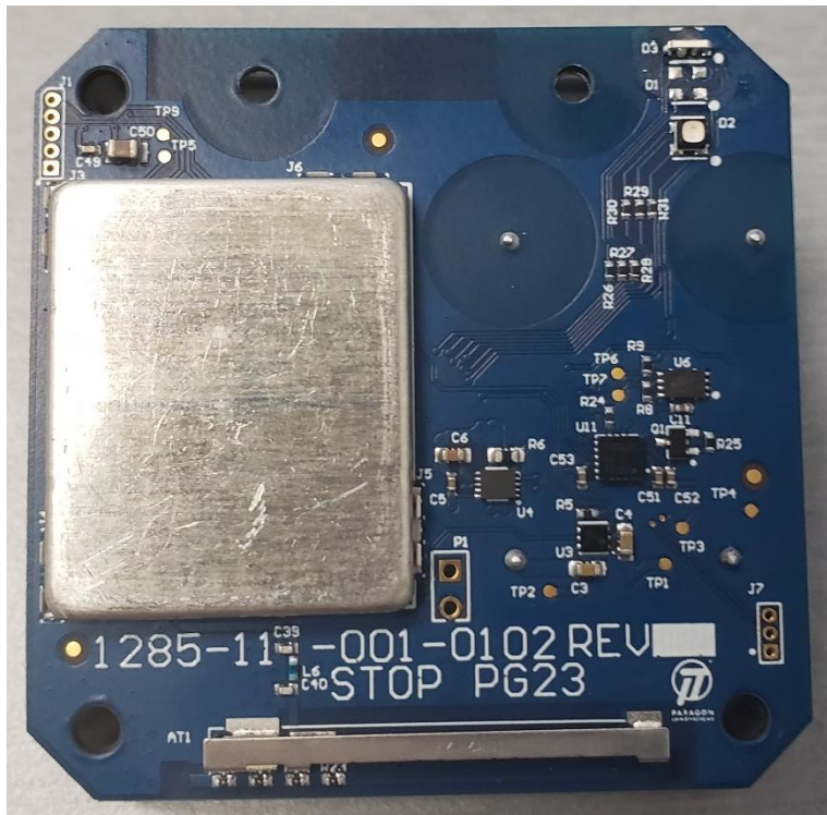
Top of BLUrepeater with Shield Installed
