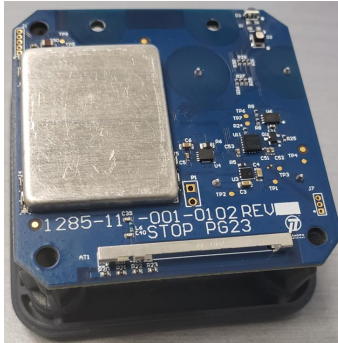
BLUrepeater V1 PCB Installed in Enclosure
