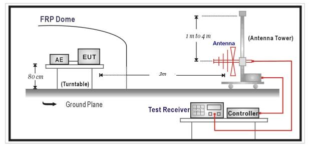
Above 1GHz Test Setup:
