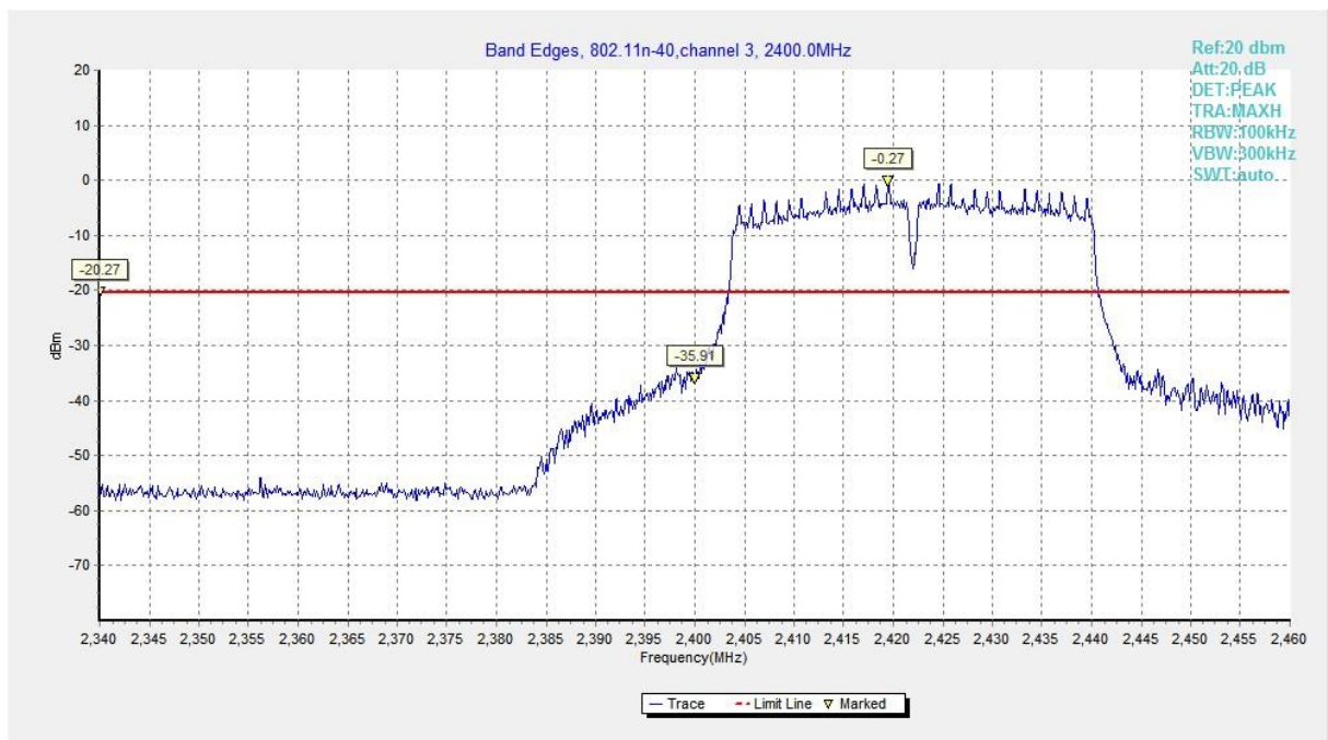
Fig.31 Band Edges (802.11n HT40, CH 3)
