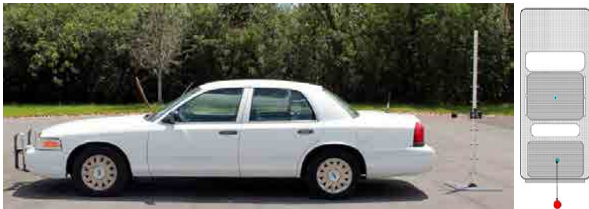
Test measurement setup for Bystander, trunk mount antenna behind vehicle
