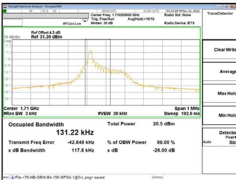
Band4-26dB/99% OBW-19952 Channel-QPSK-1@0-15K
