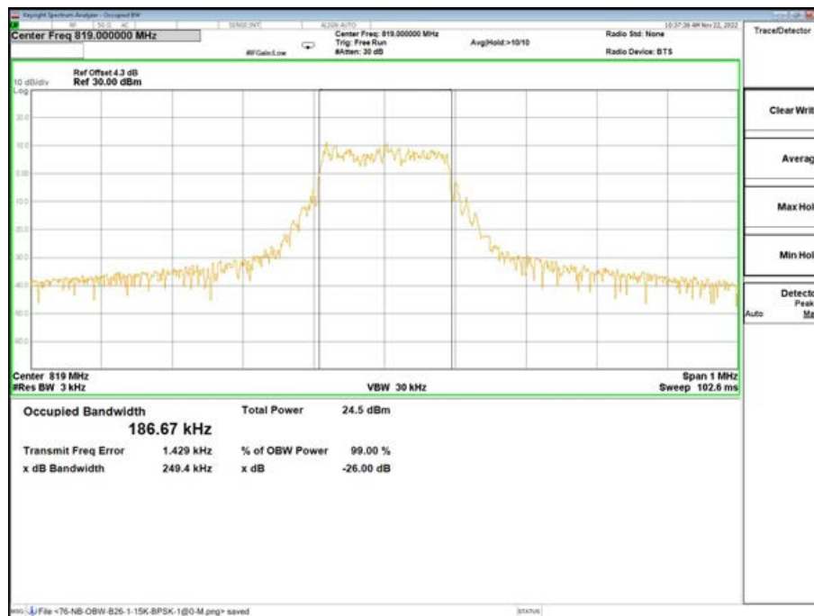
Band26-26dB/99% OBW-26740 Channel-QPSK-12@0-15K
