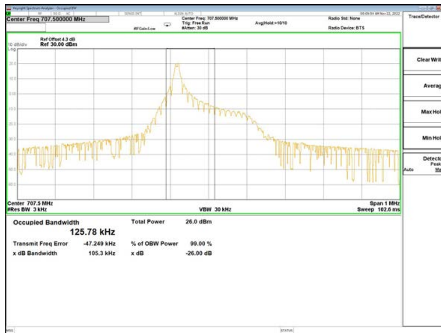
Band12-26dB/99% OBW-23095 Channel-BPSK-1@0-15K
