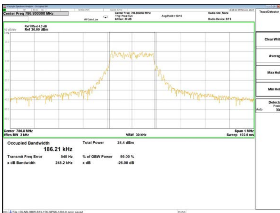
Band13-26dB/99% OBW-23278 Channel-QPSK-12@0-15K
