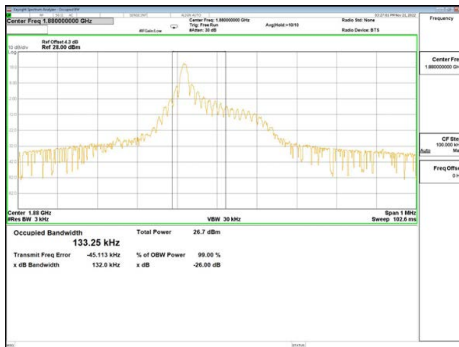
Band2-26dB/99% OBW-18900 Channel-QPSK-1@0-15K
