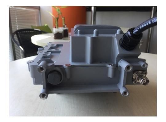
Photograph No.6 "AirSpeed1200 2.6 GHz (B41LH)" base station rear side view
