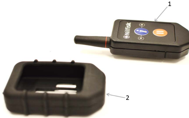
Figure 4G2. RID Removed From Cover
