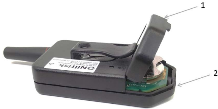
Figure 4G10. Replacing Battery Cover
