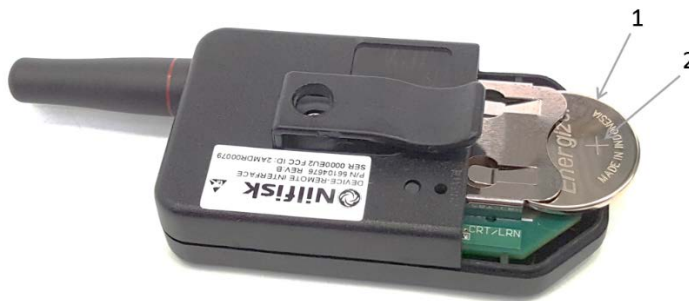
Figure 4G8. Checking RID Battery Polarity
