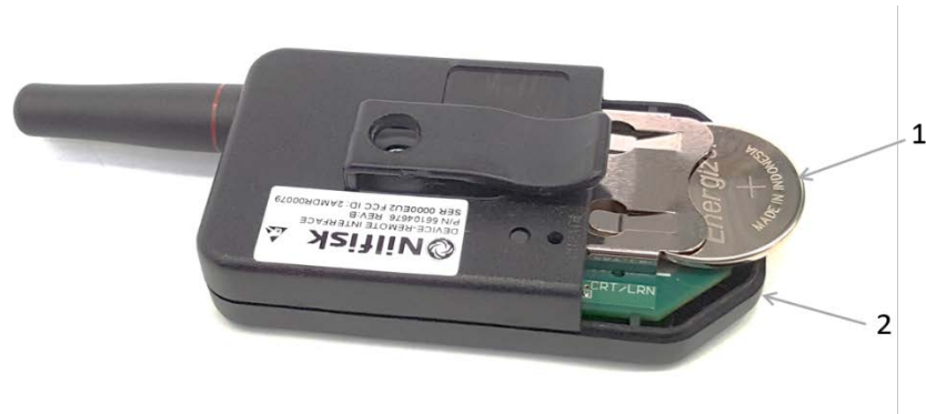
Figure 4G7. RID Final Battery Removal
