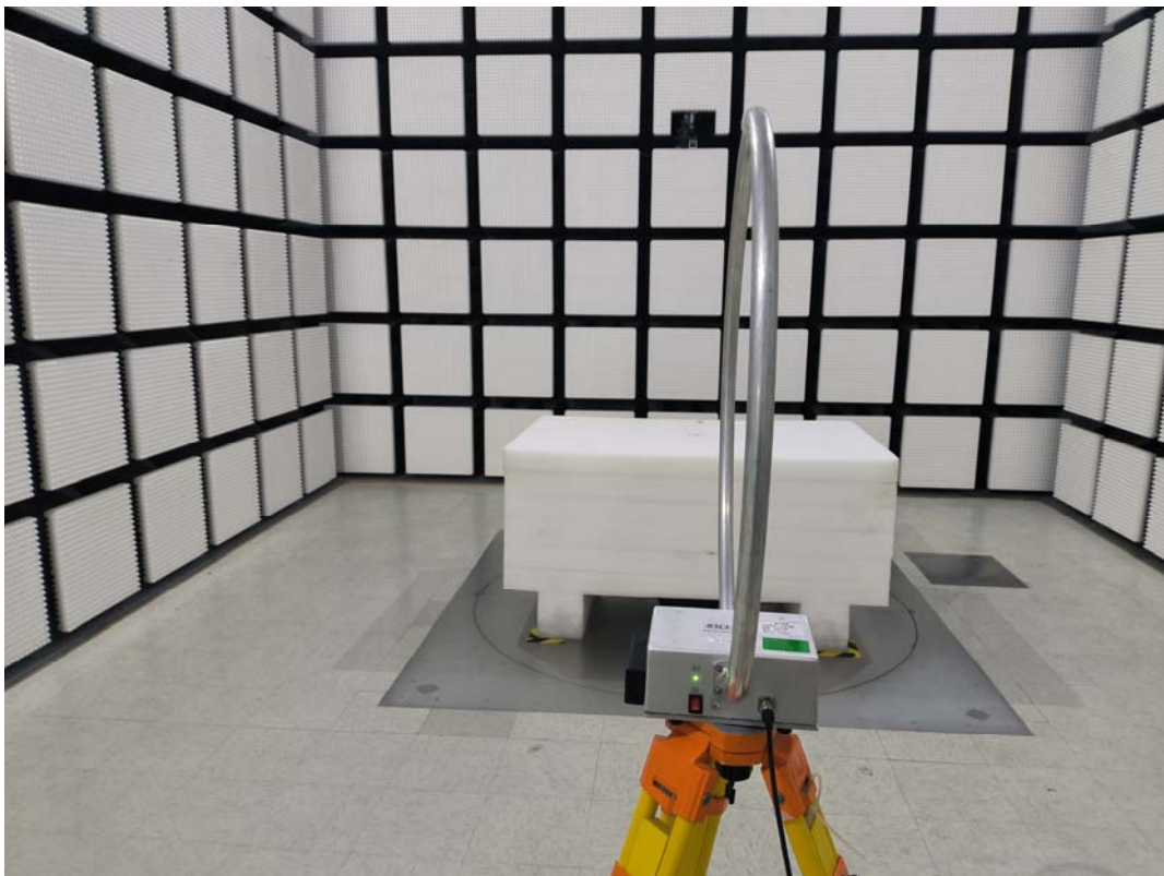
Radiated Emission 9kHz-30MHz View-Perpendicular
