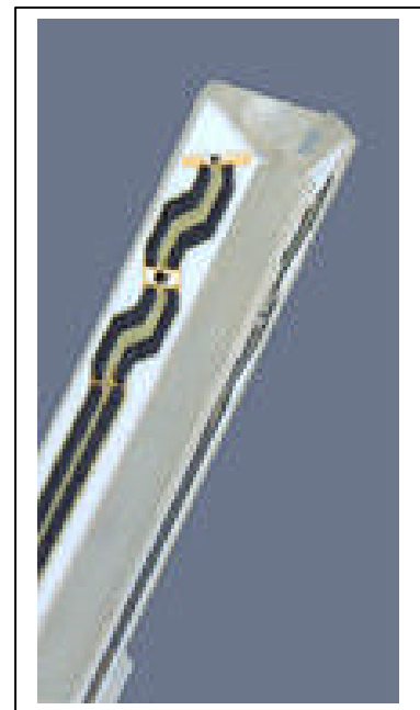
Inside view of ET3DV6 E-field Probe
