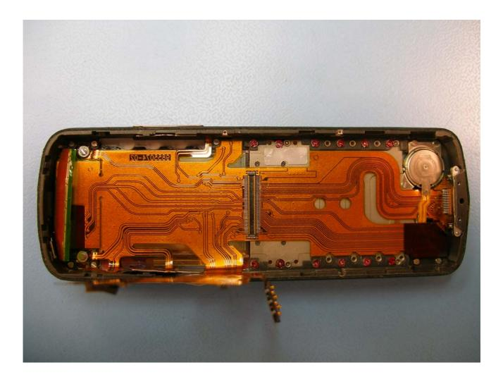
Exhibit 4: INTERNAL VIEW of Vertu FCCID: P7QRHV-2 showing reverse of display module and interconnections.
