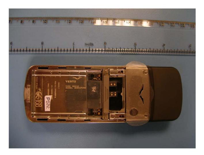
Exhibit 1: INTERNAL View of Vertu FCCID: P7QRHV-2, battery cover removed to show location of
