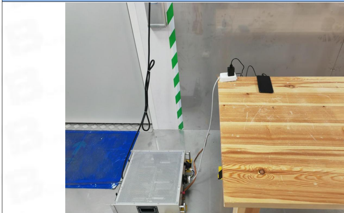
Conducted Emission at AC power line
