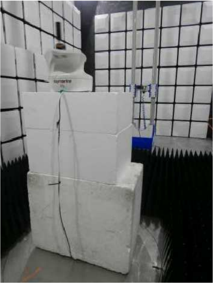
Figure 76 - Test Setup - 1 GHz to 18 GHz
