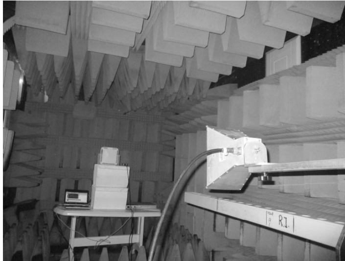
Figure 5. Radiated Emission Test 1-18GHz
