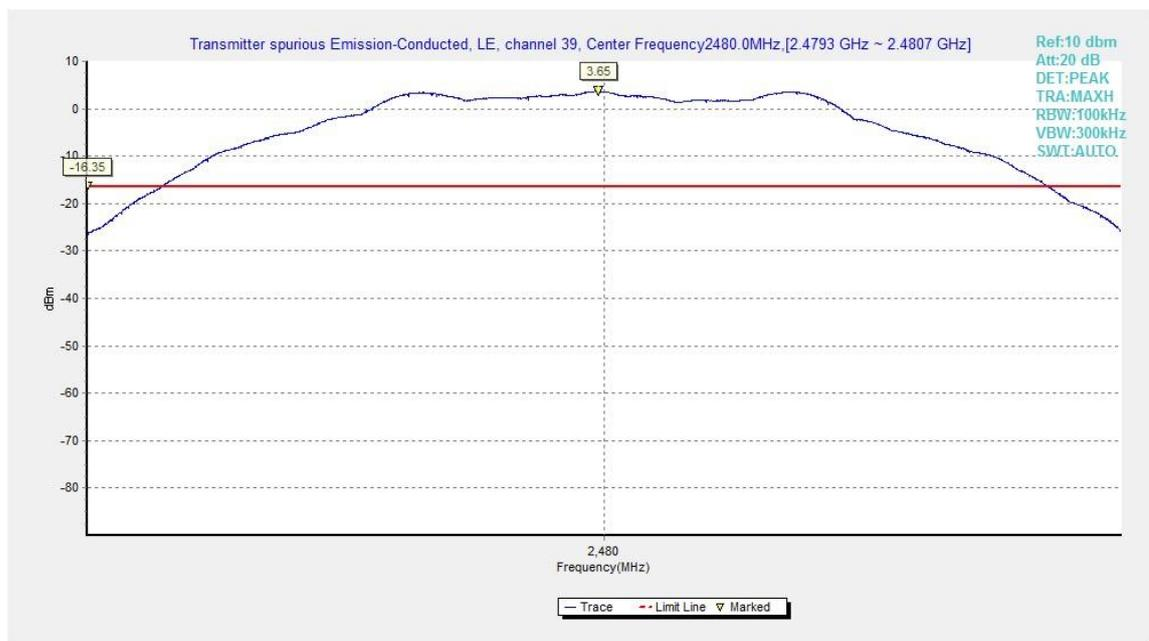
Fig.13. Transmitter Spurious Emission -Conducted: GFSK, 2480 MHz
