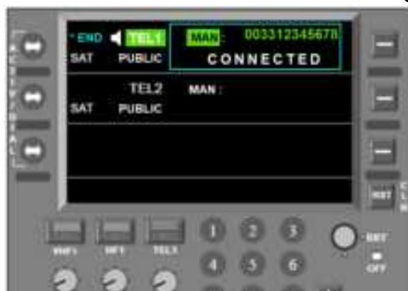
Figure 7-28: RMP - TEL Page - Outgoing Call - Connected
