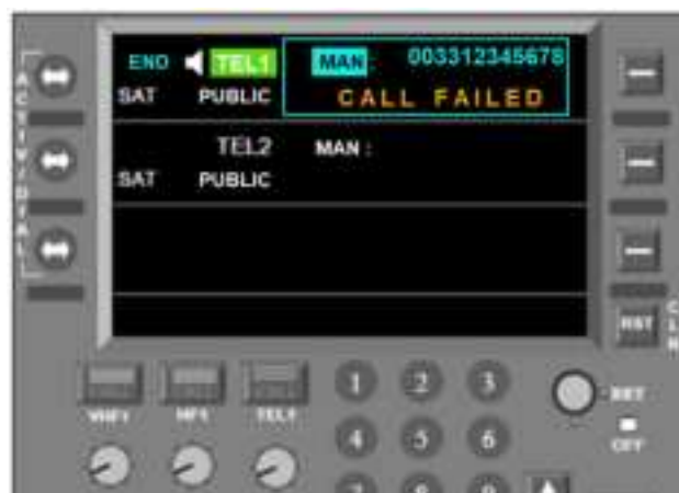
Figure 7-29: RMP - TEL Page - Outgoing Call - Call Failed
