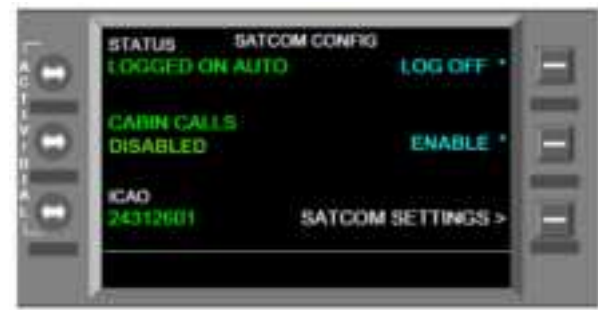
Figure 9-4: RMP - SATCOM Config - Cabin calls disabled
