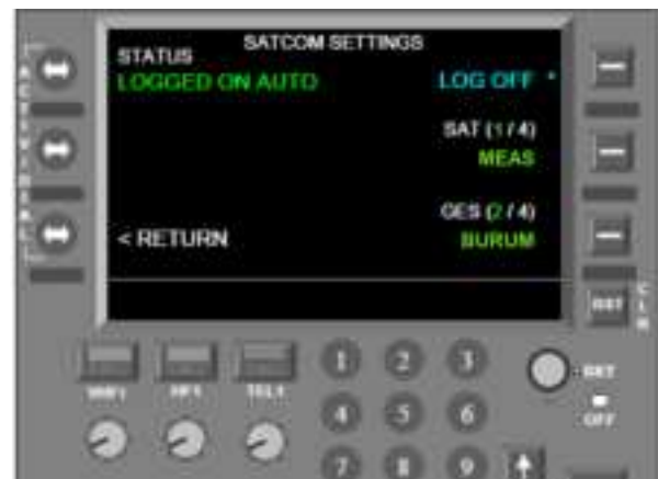
Figure 8-2: RMP - SATCOM Settings - ACARS Data Available
