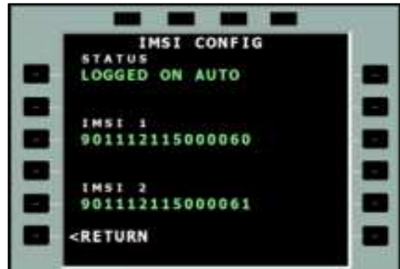
Figure 5-21: AVIATOR 700S - IMSI Config
