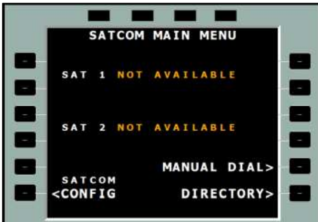
Figure 5-5: MCDU - SATCOM Main Menu - Voice Not Available
