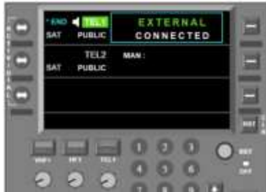
Figure 7-33: RMP - TEL Page - Incoming Call - Connected
