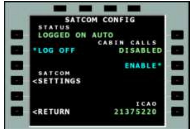
Figure 9-2: MCDU - SATCOM Config - Cabin calls disabled
