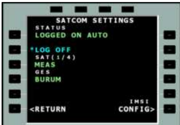
Figure 8-1: MCDU - SATCOM Settings - ACARS Data Available
