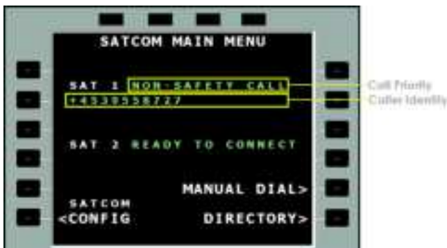
Figure 7-14: MCDU - SATCOM Main Menu - Incoming call - Unknown caller identity
