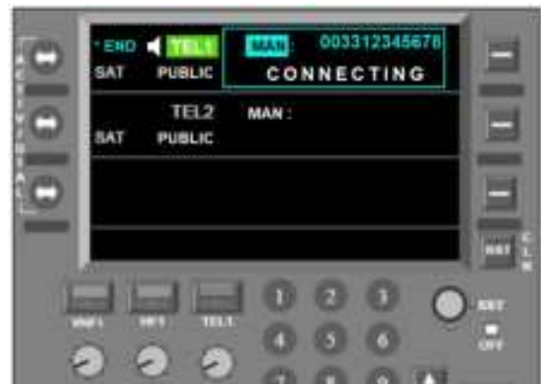
Figure 7-27: RMP - TEL Page - Outgoing Call – Connecting
