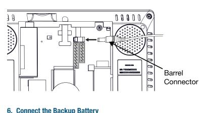
Align pins, then carefully insert the battery cable.
