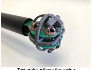
Test probe, without the casing
