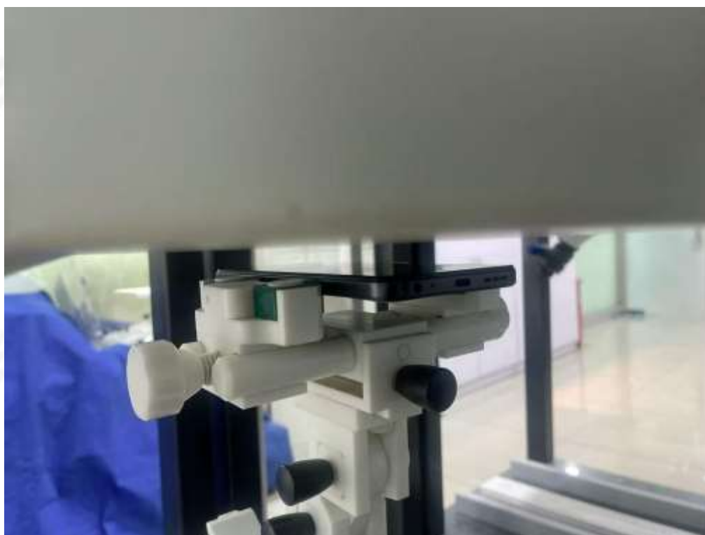
Body Front side(separation distance is 10mm)
