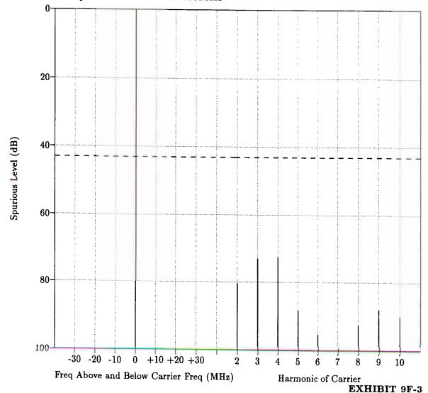
TRANSMITTER SPURIOUS EMISSION CHARACTERISTIC CONDUCTED SPURIOUS and HARMONIC EMISSIONS
