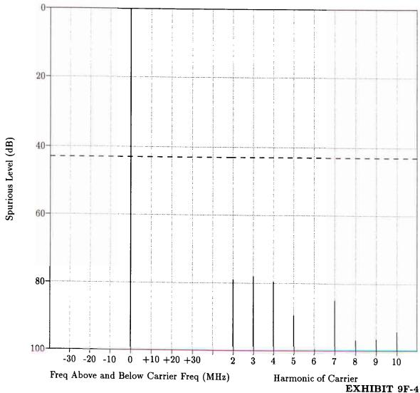
TRANSMITTER SPURIOUS EMISSION CHARACTERISTIC RADIATED SPURIOUS and HARMONIC EMISSIONS
