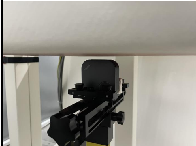
Left Side of EUT with 0.5 cm Gap
