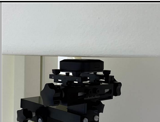
Rear Face of EUT with 0.5 cm Gap
