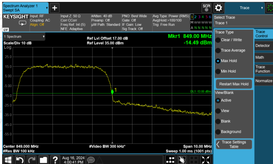
Higher Band Edge Plot on Channel 4233
